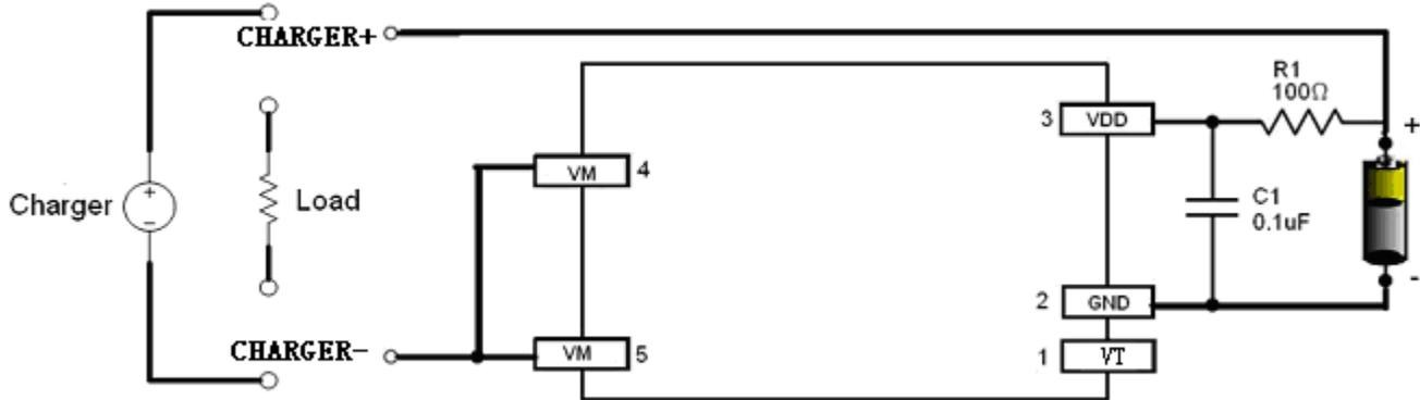
**Fig 6 XB5350G in a Typical Battery Protection Circuit**
