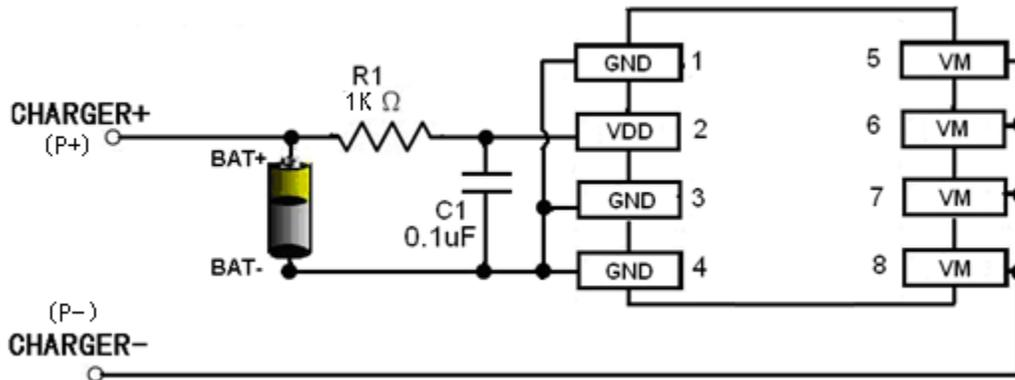
Fig 6 XB8608A2 in a Typical Battery Protection Circuit
