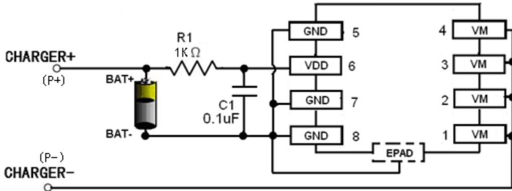
**Fig 6 XB8889A in a Typical Battery Protection Circuit**
