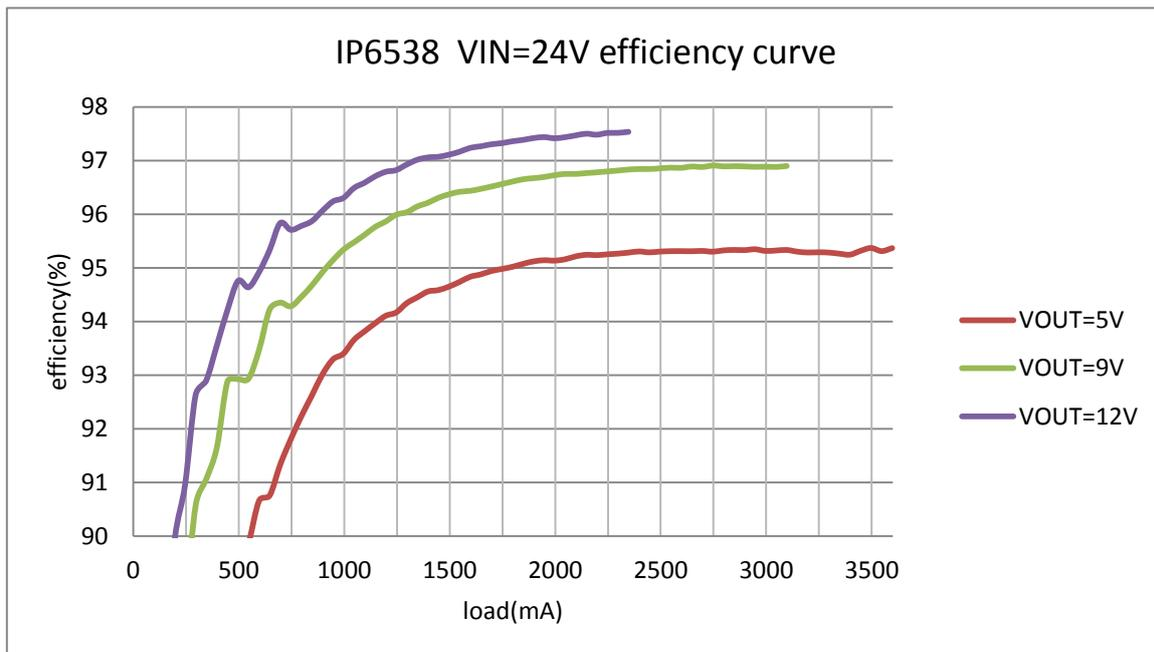
Figure 3. IP6538 output efficiency curve when  $V_{IN} = 24V$
