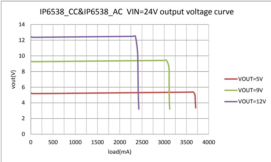
Figure 4. IP6538\_CC and IP6538\_AC Vout-lout curve when VIN=24V
