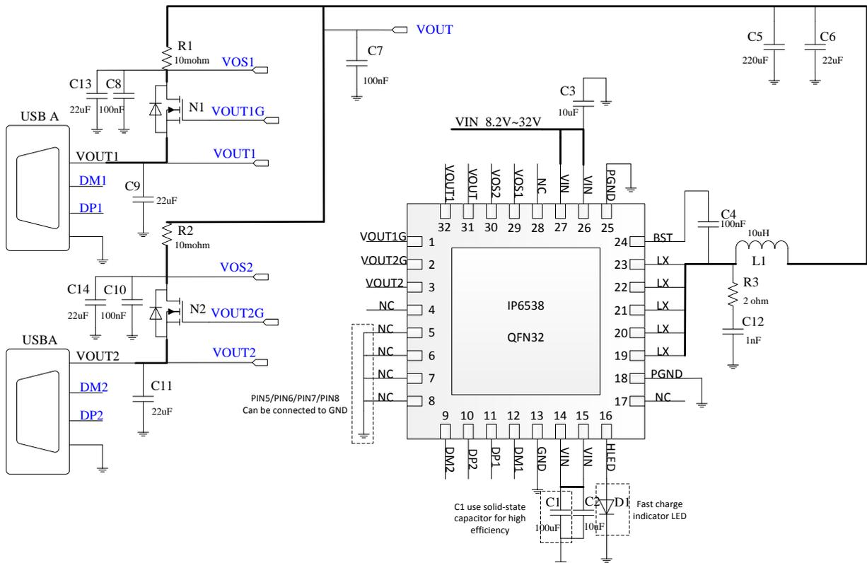
Figure 8. IP6538\_AA dual USB A output ports fast charge application schematic diagram
