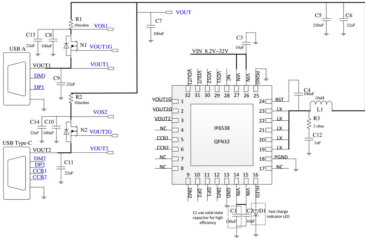
Figure 7. IP6538\_AC USB A plus USB Type-C output ports fast charge application schematic diagram
