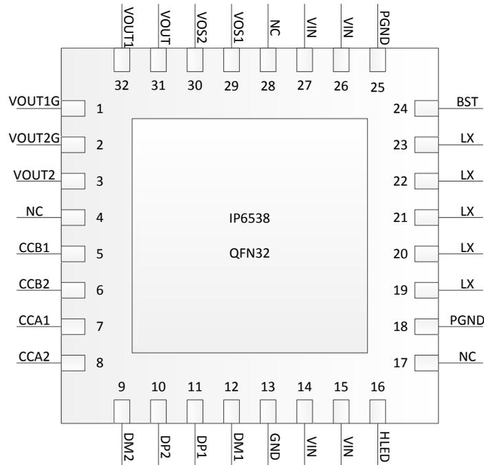
Figure 2. Pin Functions
