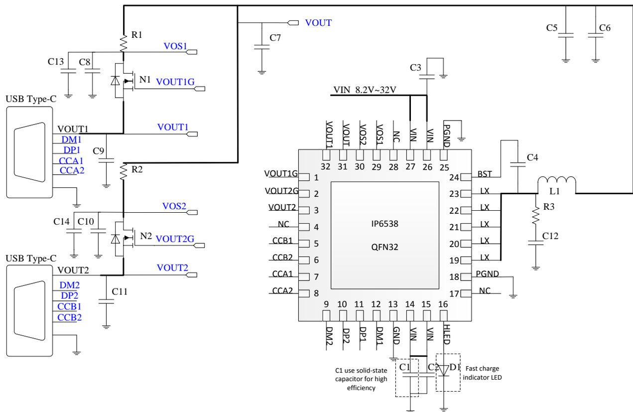
Figure 1. IP6538\_CC dual USB Type-C output ports simplified application schematic diagram
