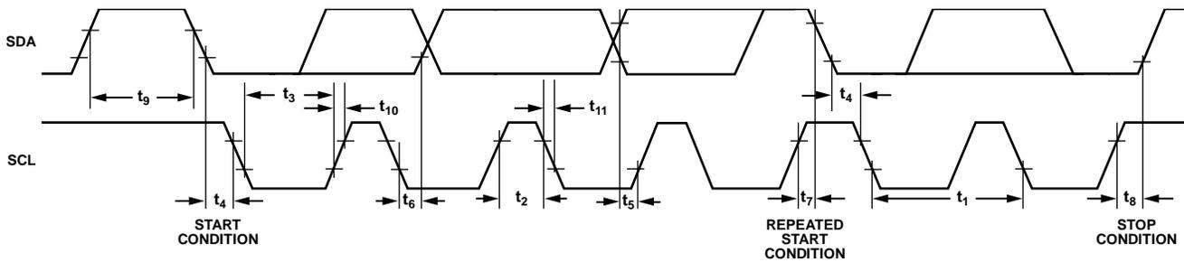
Figure 29. I<sup>2</sup>C Timing Diagram
