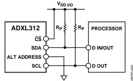
Figure 27. I<sup>2</sup>C Connection Diagram (Address 0x53)
