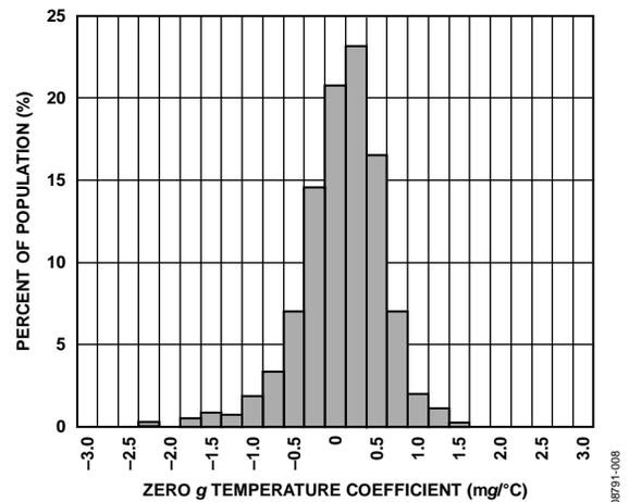
Figure 8. Z-Axis Zero-g Bias Drift,  $V_S = V_{DD/IO} = 3.3 V$
