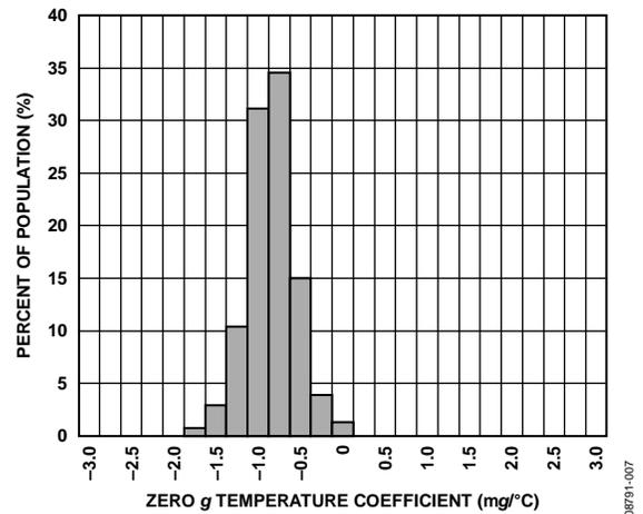
Figure 7. Y-Axis Zero-g Bias Drift,  $V_S = V_{DD/IO} = 3.3 V$
