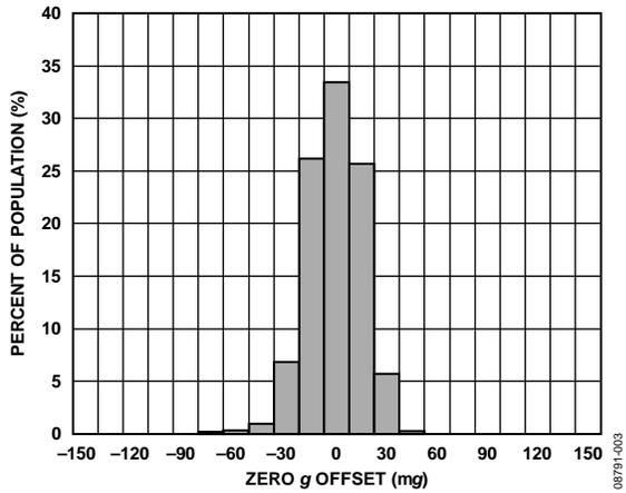
Figure 3. X-Axis Zero-g Bias, 25°C,  $V_S = V_{DD/IO} = 3.3 V$
