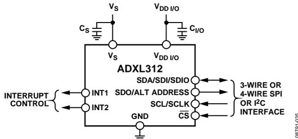
Figure 31. Application Diagram
