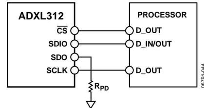
Figure 21. 3-Wire SPI Connection Diagram
