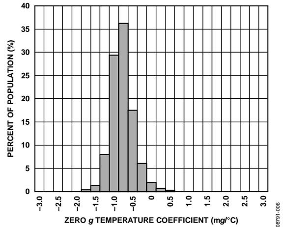
Figure 6. X-Axis Zero-g Bias Drift,  $V_S = V_{DD/IO} = 3.3 V$
