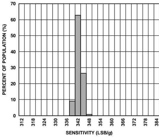
Figure 9. X-Axis Sensitivity,  $V_S = V_{DD/IO} = 3.3\text{ V}$ ,  $25^\circ\text{C}$
