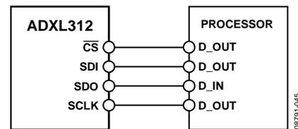
Figure 22. 4-Wire SPI Connection Diagram
