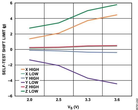
Figure 30. Self-Test Output Change Limits vs. Supply Voltage
