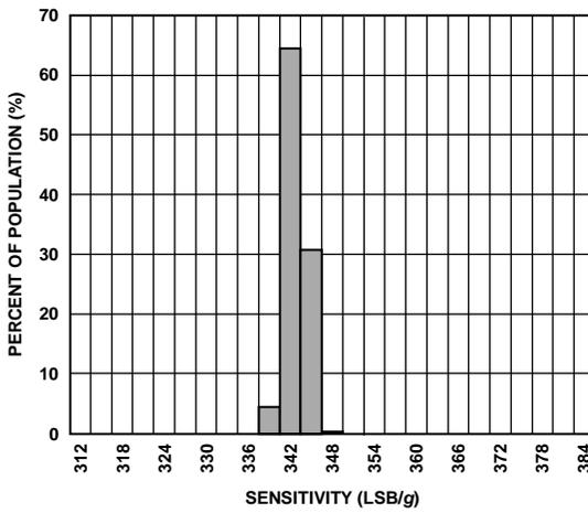
Figure 11. Z-Axis Sensitivity,  $V_S = V_{DD/IO} = 3.3\text{ V}$ ,  $25^\circ\text{C}$
