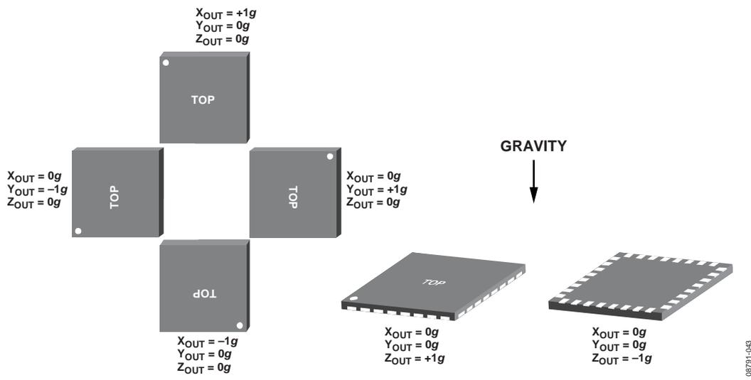
Figure 38. Output Response vs. Orientation to Gravity
