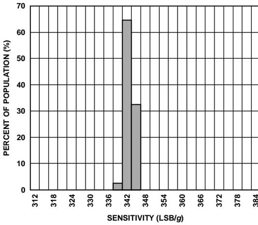
Figure 10. Y-Axis Sensitivity,  $V_S = V_{DD/IO} = 3.3\text{ V}$ ,  $25^\circ\text{C}$
