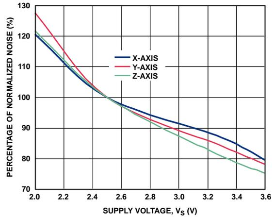
Figure 36. Normalized Noise vs. Supply Voltage,  $V_S$
