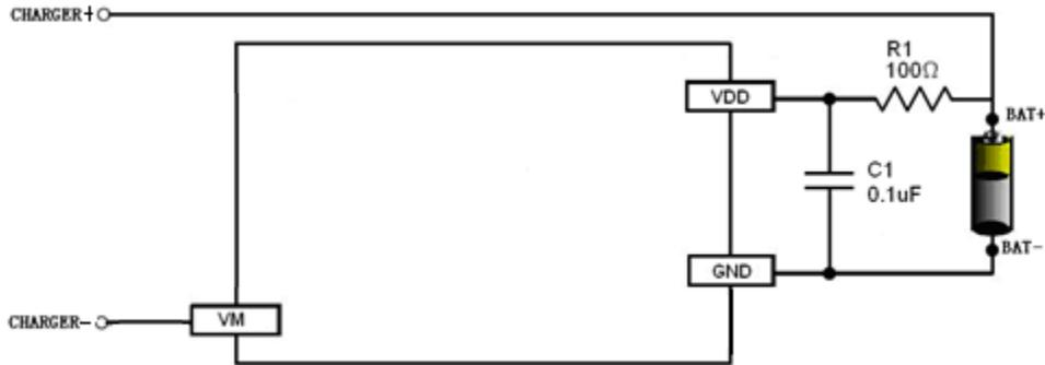
**Fig 6 XB3153IS in a Typical Battery Protection Circuit**
