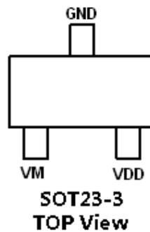
Figure 2. PIN Configuration
