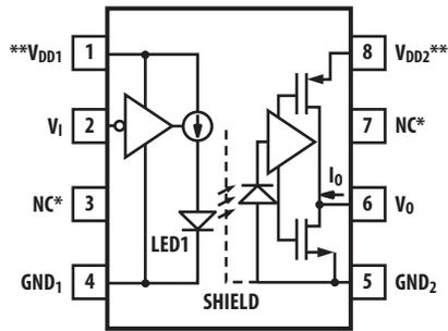
\* Pin 3 is multiplexed as a test pin that can connect to  $V_{DD}$  or left unconnected. Pin 7 is not connected internally.
