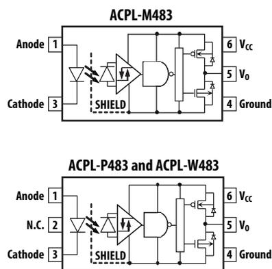
Note: A 0.1  $\mu\text{F}$  bypass capacitor must be connected between pins 4 and 6. Truth Table Guaranteed:  $V_{CC}$  from 4.5V to 30V.
