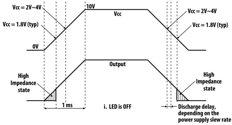
**Figure 11 V<sub>CC</sub> Ramp When LED OFF**
