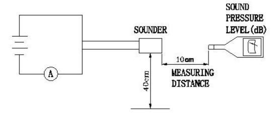
2. In the measuring test, buzzer is placed as follows
