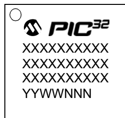
64-Lead QFN (9x9x0.9 mm)
