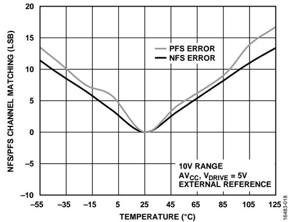
Figure 7. NFS and PFS Channel Matching vs. Temperature
