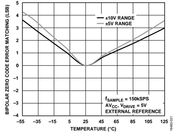
Figure 9. Channel to Channel Bipolar Zero Code Error Matching vs. Temperature
