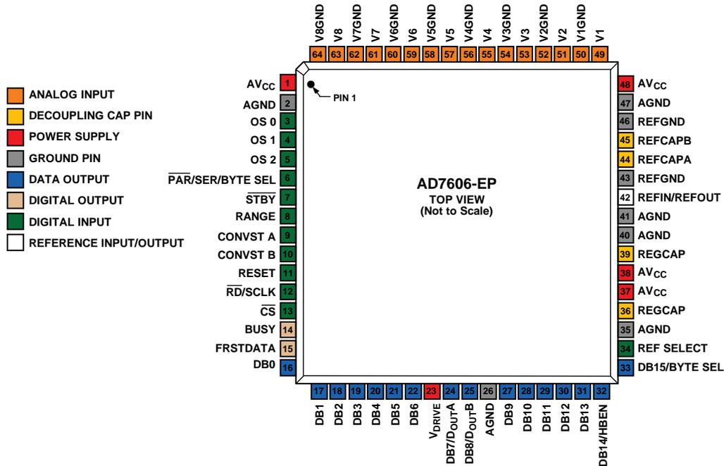
Figure 4. Pin Configuration
