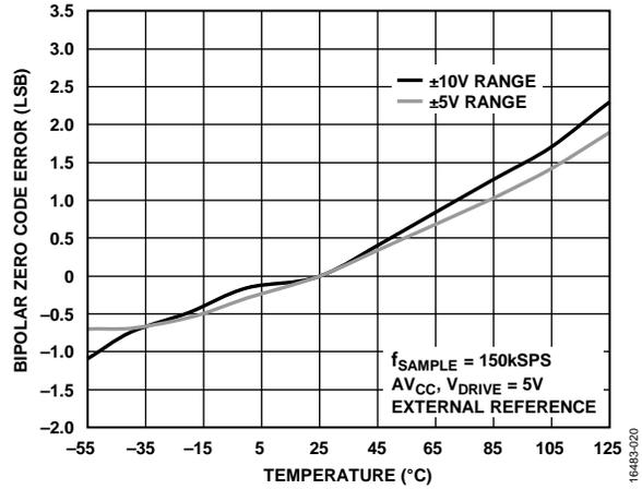
Figure 8. Bipolar Zero Code Error vs. Temperature
