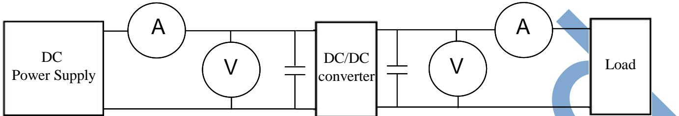
◎DC Power Supply: It offers a wide voltage and current range precisely.
