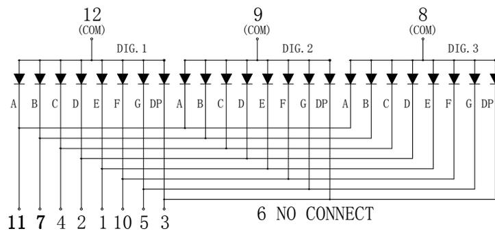
Internal Circuit Diagram (Common Cathode)
