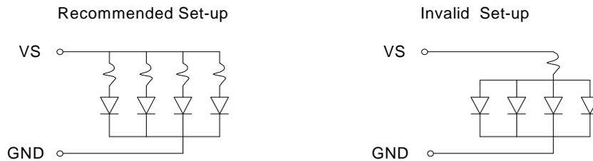
3. The driving circuit should be designed to protect the LED against reverse voltages and transient voltage spikes when the circuit is powered up or shut down.
