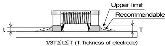
Accordingly increasing the solder volume, the mechanical stress to Chip is also increased. Exceeding solder volume may cause the failure of mechanical or electrical performance.
