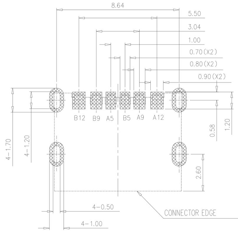
RECOMMENDED PCB LAYOUT (TOP VIEW)
