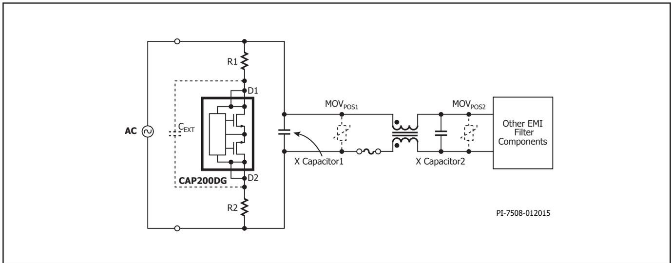
Figure 4. Placement Options of MOV and C<sub>EXT</sub>.
