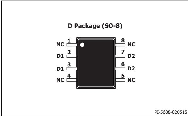
Figure 3. Pin Configuration.
