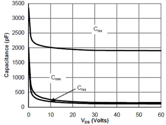
Figure 8: Capacitance Characteristics
