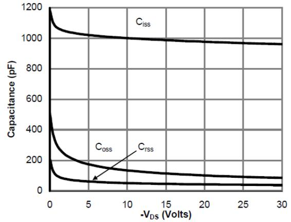
Figure 8: Capacitance Characteristics
