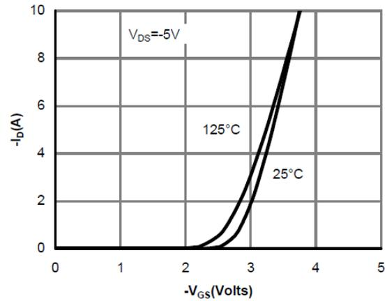
Figure 2: Transfer Characteristics
