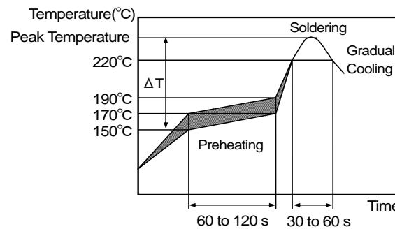
[Allowable Reflow Soldering Temperature and Time]
