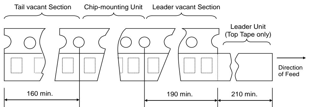
5. Accumulate tolerance of sprocket holes pitch =  $+\/-0.3\text{mm}/10\text{ pitch}$
