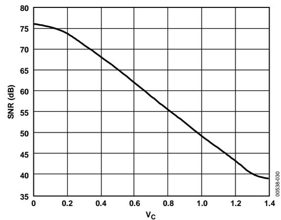
Figure 32. SNR vs. Control Voltage—Low Ripple Mode
