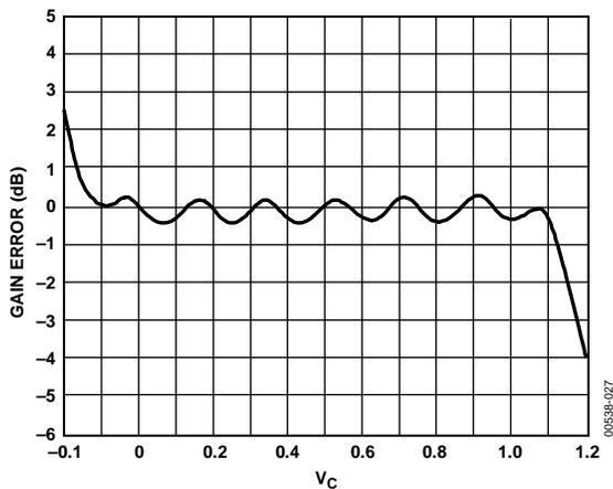
Figure 29. Gain Error for Cascaded Stages—Parallel Control
