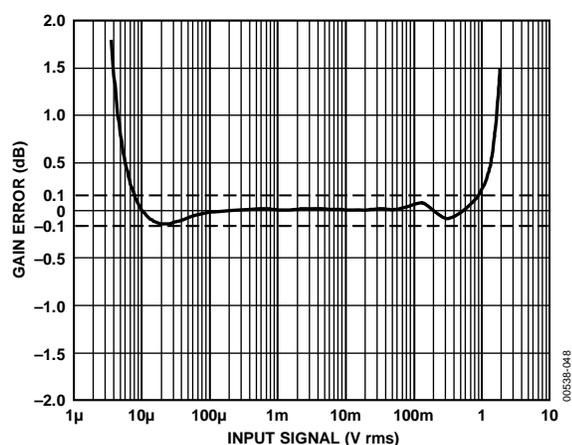
Figure 50. Adding the 2 dB Offsets Improves the Linearization
