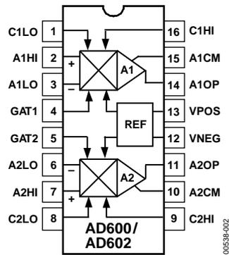
Figure 2. Pin Configuration
