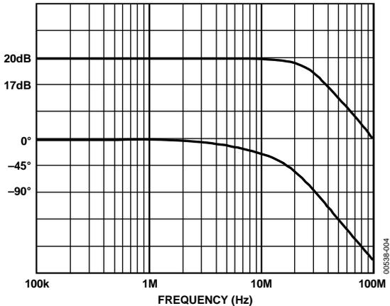
Figure 4. AD600 Frequency and Phase Response vs. Gain
