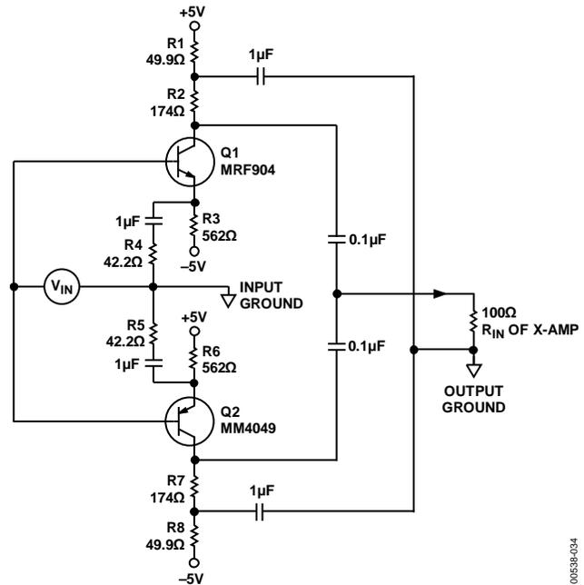
Figure 36. A Low Noise Preamplifier for the AD600/AD602
