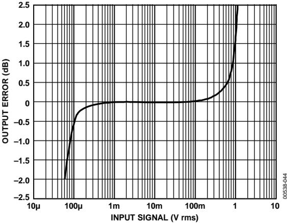
Figure 46. Using a 3 dB Offset Network Reduces Ripple
