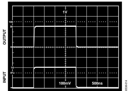
Figure 14. Transient Response, Medium and High Gain
