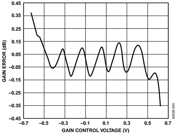
Figure 3. Gain Error vs. Gain Control Voltage
