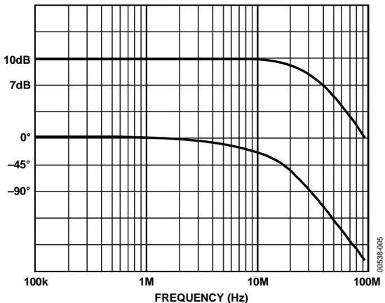
Figure 5. AD602 Frequency and Phase Response vs. Gain
