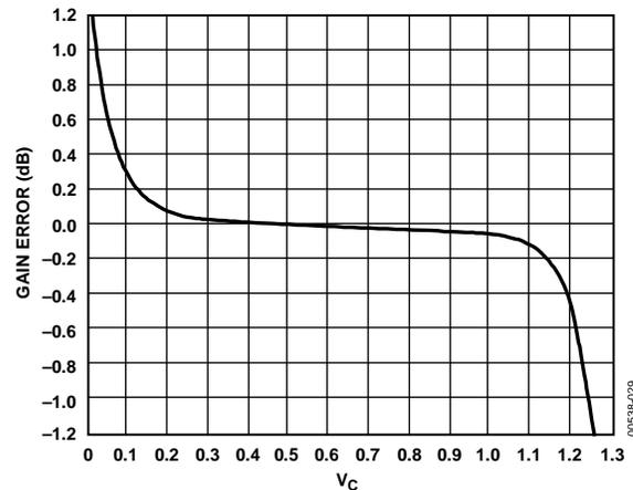
Figure 31. Gain Error for Cascaded Stages—Low Ripple Mode
