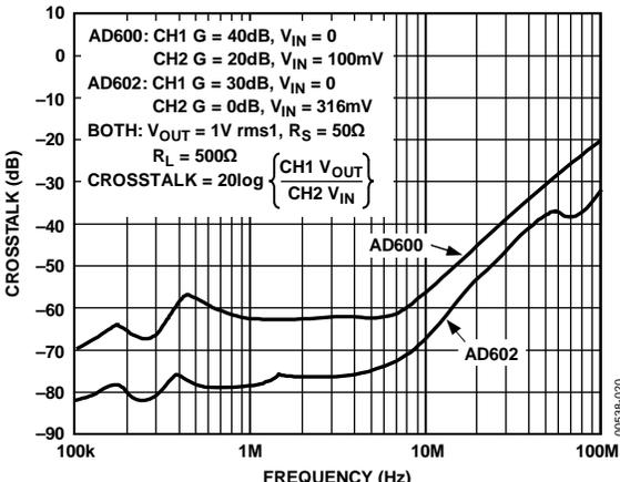
Figure 20. Crosstalk Between A1 and A2 vs. Frequency
