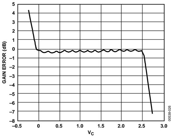
Figure 28. Gain Error for Cascaded Stages—Sequential Control
