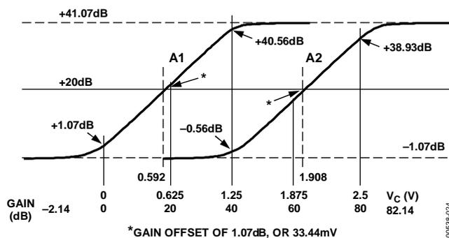
Figure 26. Explanation of Offset Calibration for Sequential Control
