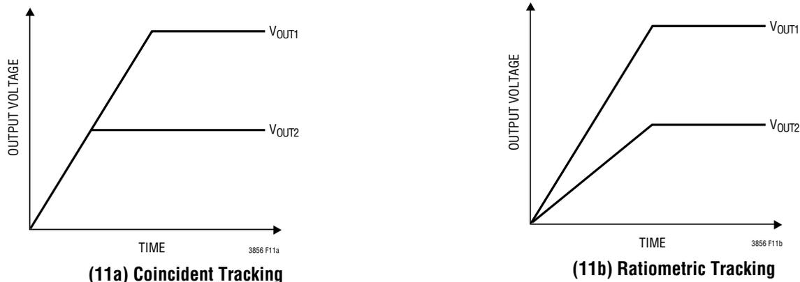
Figure 11. Two Different Modes of Output Voltage Tracking
