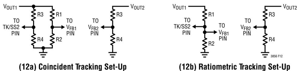
Figure 12. Set-Up and Coincident and Ratiometric Tracking
