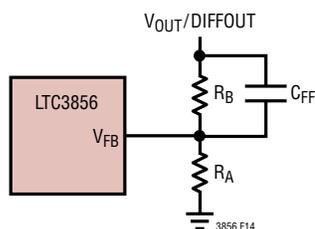
Figure 14. Setting Output Voltage without the DIFFAMP
