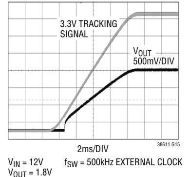
**Start-Up Response Into a 300mV Prebiased Output (Single Phase Using FDMF6707B DrMOS)**
