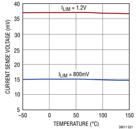
**I<sub>LIM</sub> Pin Current vs Temperature**
