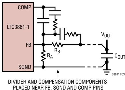
Figure 3. Output Divider and Compensation Component Placement
