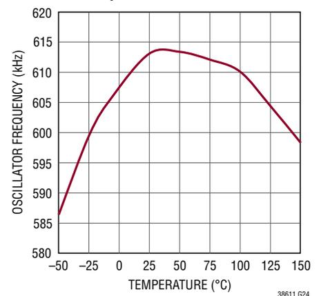
**400kHz Preset Frequency vs Temperature**
