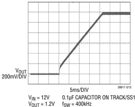
**Coincident Tracking (Single Phase Using FDMF6707B DrMOS)**
