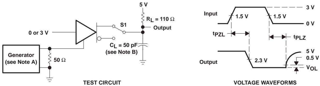
NOTES: A. The input pulse is supplied by a generator having the following characteristics: PRR = 1.25 kHz, 50% duty cycle,  $t_r \leq 10$  ns,  $t_f \leq 10$  ns,  $Z_O = 50 \Omega$ .
