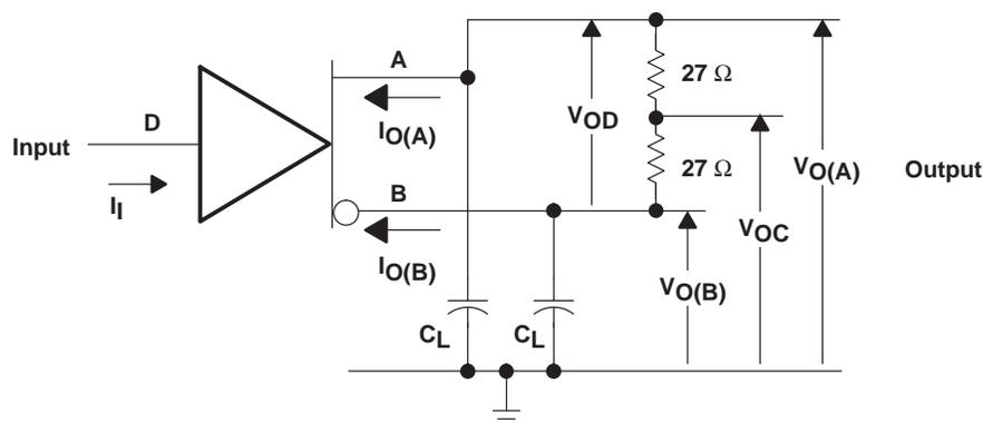
NOTES: A. Resistance values are in ohms and are 1% tolerance.
