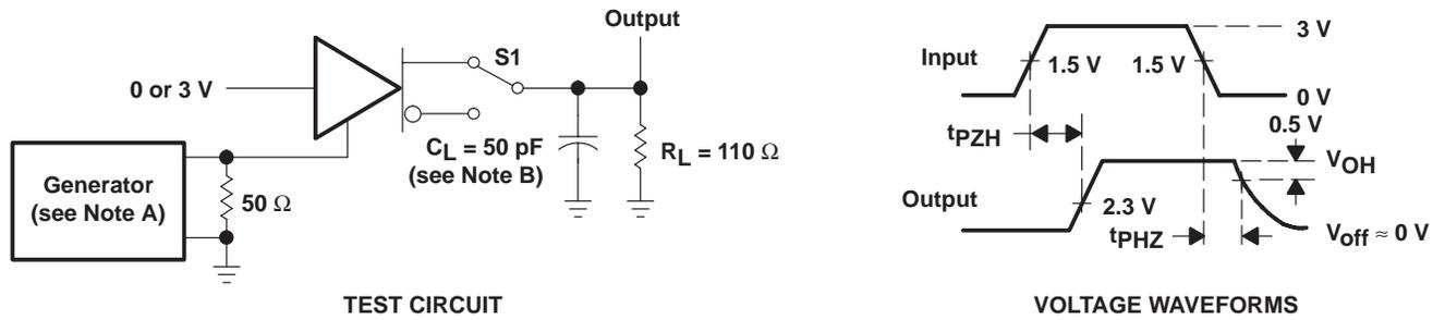
NOTES: A. The input pulse is supplied by a generator having the following characteristics: PRR = 1.25 kHz, 50% duty cycle,  $t_r \leq 10$  ns,  $t_f \leq 10$  ns,  $Z_O = 50 \Omega$ .
