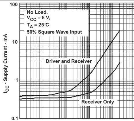
**Figure 4. 65HVD3088E RMS Supply Current versus Signal Rate**
