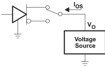
Figure 14. Driver Short-Circuit
