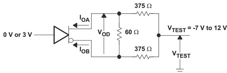
**Figure 9. Driver Test Circuit,  $V_{OD}$  With Common-Mode Loading**
