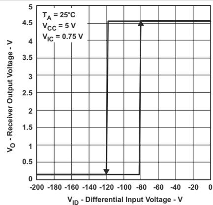
**Figure 6. Receiver Output Voltage versus Differential Input Voltage**
