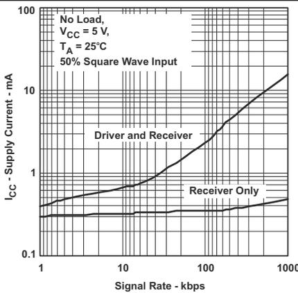
**Figure 3. 65HVD3085E RMS Supply Current versus Signaling Rate**
