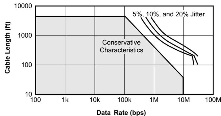
**Figure 24. Cable Length vs Data Rate Characteristic**
