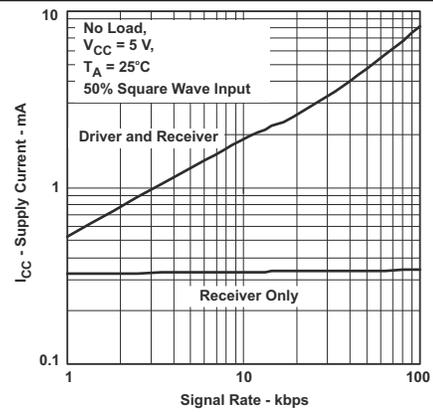
**Figure 2. 65HVD3082E RMS Supply Current versus Signaling Rate**
