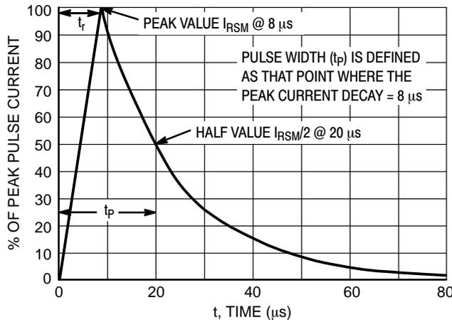
Figure 13. 8 X 20 μs Pulse Waveform
