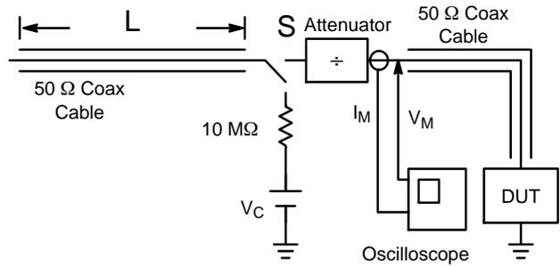
**Figure 14. Simplified Schematic of a Typical TLP System**
