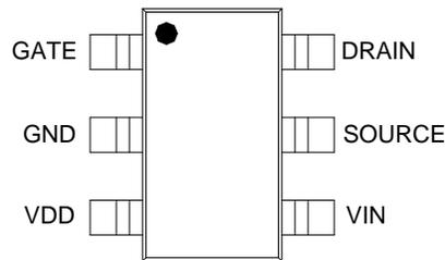
Figure 4. Pin Configuration
