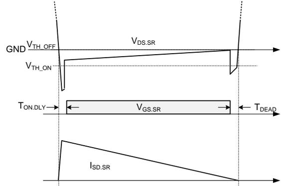
**Figure 5. SR MOSFET Operation Waveforms (Ideal Case)**
