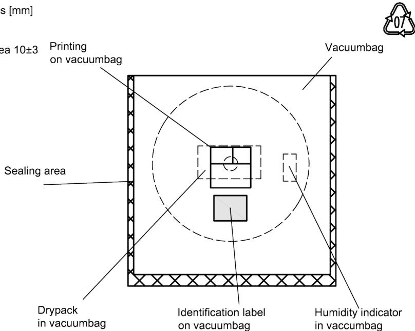
**Figure 19:** Drawing of moisture barrier bag (MBB) for reel with diameter of 330 mm.
