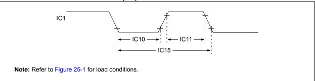
TABLE 25-27: INPUT CAPTURE 1 MODULE TIMING REQUIREMENTS
