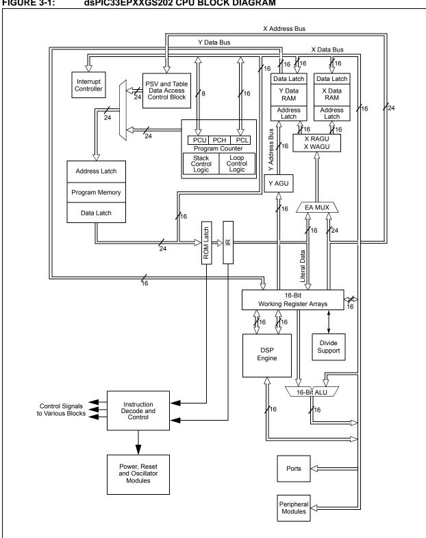
FIGURE 3-1: dsPIC33EPXXGS202 CPU BLOCK DIAGRAM
