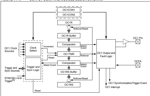
Note 1: The trigger/sync source is enabled by default and is set to Timer2 as a source. This timer must be enabled for OC1 module operation or the trigger/sync source must be changed to another source option.
