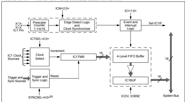
Note 1: The trigger/sync source is enabled by default and is set to Timer3 as a source. This timer must be enabled for proper IC1 module operation or the trigger/sync source must be changed to another source option.
