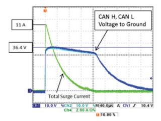
Figure 1 -CDSOT23-T24CAN Clamp Voltages for a +500 V Surge
