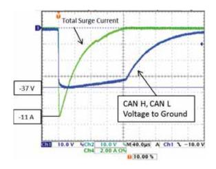
Figure 2 - CDSOT23-T24CAN Clamp Voltages for a -500 V Surge
