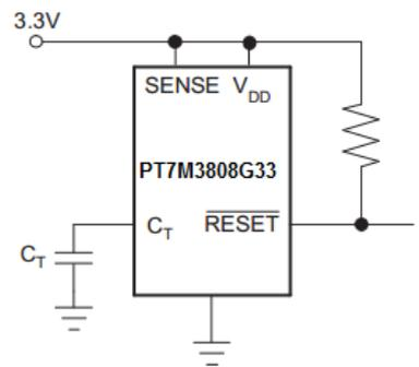
$$\text{Delay (s)} = \frac{C_T \text{ (nF)}}{175} + 0.5 \times 10^{-3} \text{ (s)}$$
