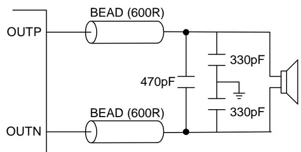
Figure 6. Typical ferrite chip bead output filter
