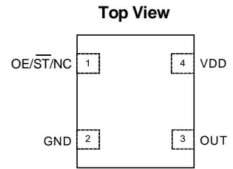
**Figure 1. Pin Assignments**
