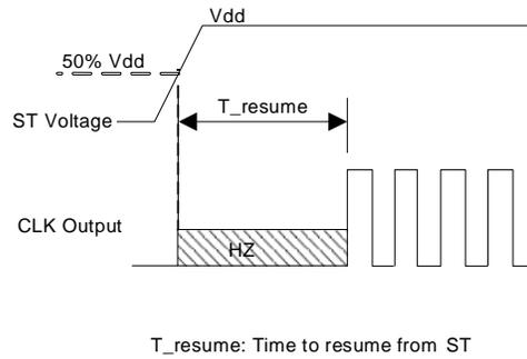
**Figure 5. Standby Resume Timing (ST Mode Only)**
