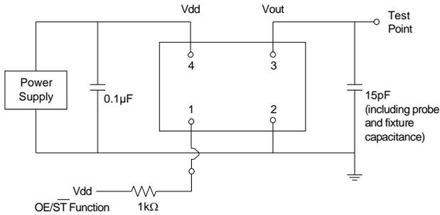
**Figure 2. Test Circuit**
