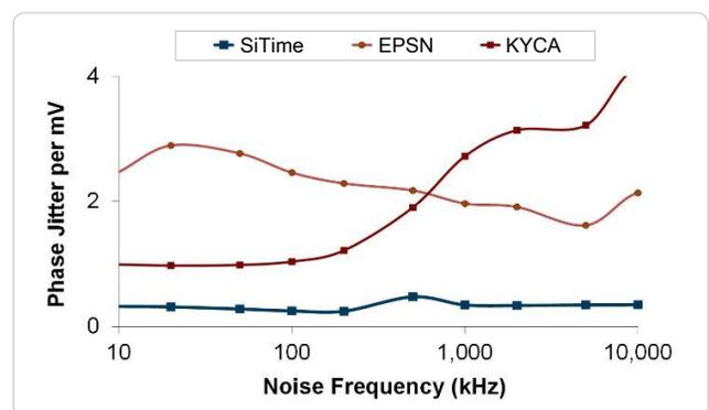
Figure 4. Power Supply Noise Rejection<sup>[4]</sup>
