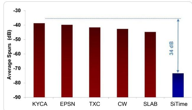
Figure 3. Electro Magnetic Susceptibility (EMS)<sup>[3]</sup>
