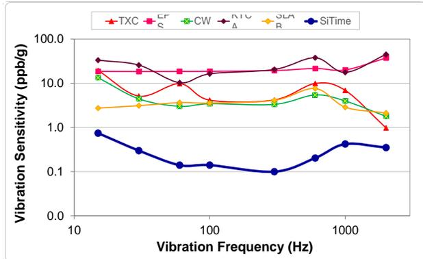
Figure 5. Vibration Robustness<sup>[5]</sup>
