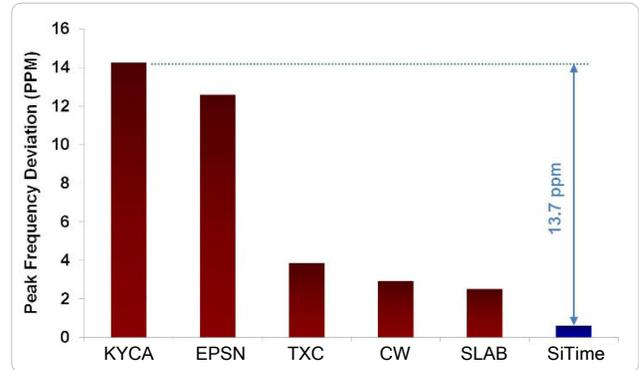
Figure 6. Shock Robustness<sup>[6]</sup>
