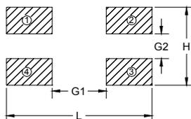
PC board should be designed so that products can prevent damage from mechanical stress when warping the board. Products shall be positioned in the sideways direction against the mechanical stress to prevent failure.
