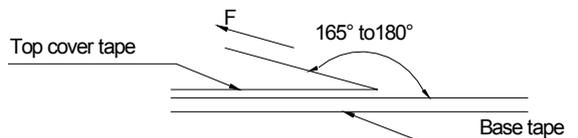
The force for tearing off cover tape is 15 to 80 grams in the arrow direction under the following conditions.
