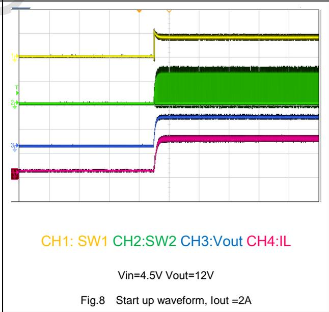
Fig.8 Start up waveform, Iout =2A
