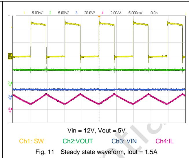
Fig. 11 Steady state waveform, Iout = 1.5A
