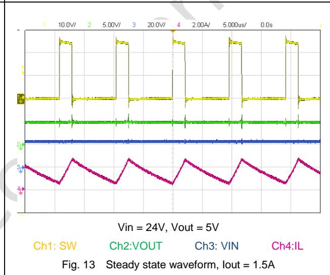
Fig. 13 Steady state waveform, Iout = 1.5A
