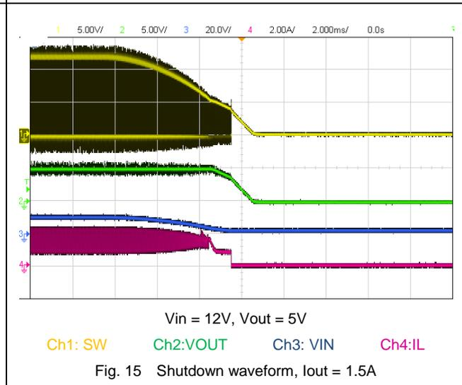
Fig. 15 Shutdown waveform, Iout = 1.5A
