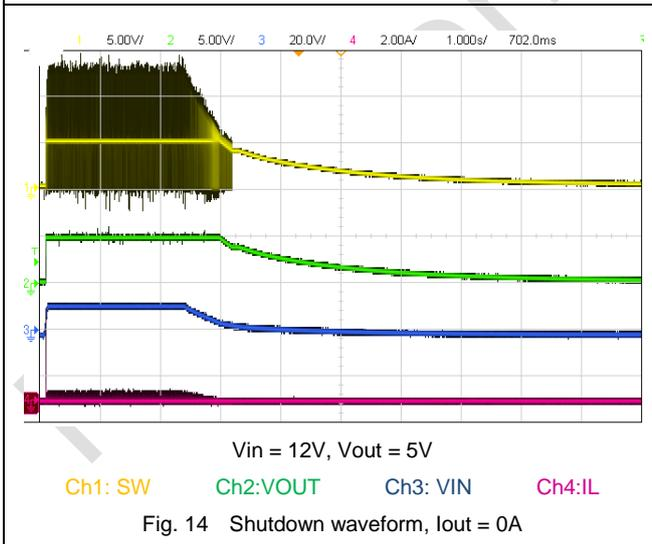
Fig. 14 Shutdown waveform, Iout = 0A
