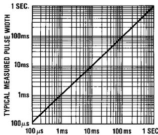
FIGURE 11. Typical Pulse Width Versus Timing RC Product
