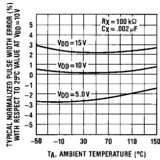
FIGURE 9. Typical Pulse Width Error Versus Temperature
