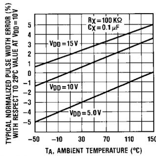
FIGURE 10. Typical Pulse Width Error Versus Temperature
