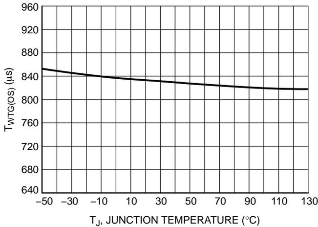
Figure 37. Watchdog Timer in "Overstress" Situation vs. Temperature
