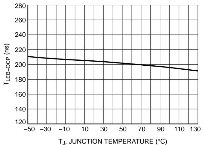
Figure 28. Over-current Protection Leading Edge Blanking vs. Temperature
