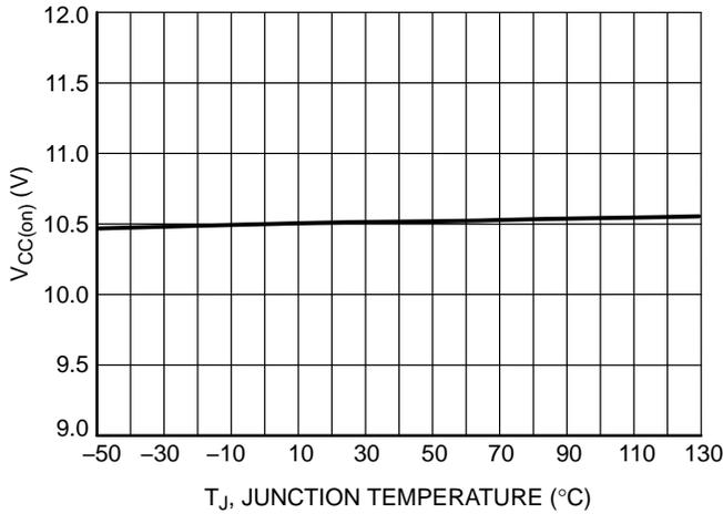
Figure 5. Start-up Threshold, V<sub>CC</sub> Increasing (V<sub>CC(on)</sub>) vs. Temperature (A, A1, A2 and A3 Versions)
