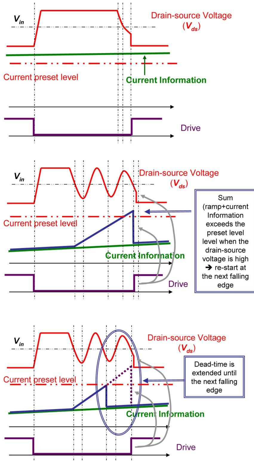
Top: CrM operation when the current information exceeds the preset level during the demagnetization phase
