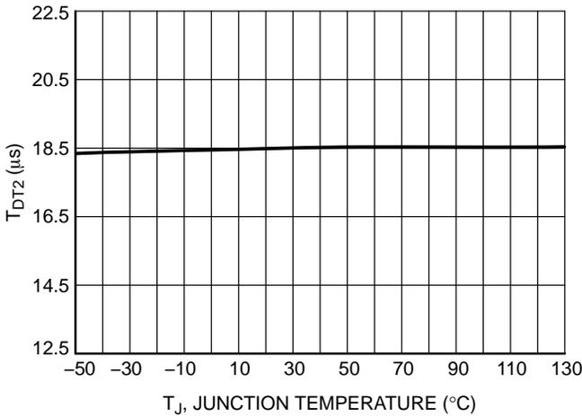
Figure 13. Dead-time,  $V_{FFcontrol} = 1.75\text{ V}$  vs. Temperature
