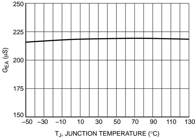
Figure 23. Error Amplifier Transconductance Gain vs. Temperature
