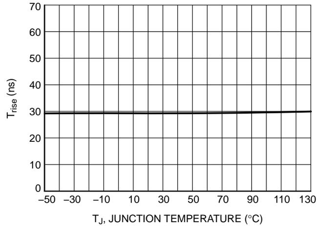
Figure 18. DRV Voltage Rise-time (C<sub>L</sub> = 1 nF, 10–90% of Output Signal) vs. Temperature
