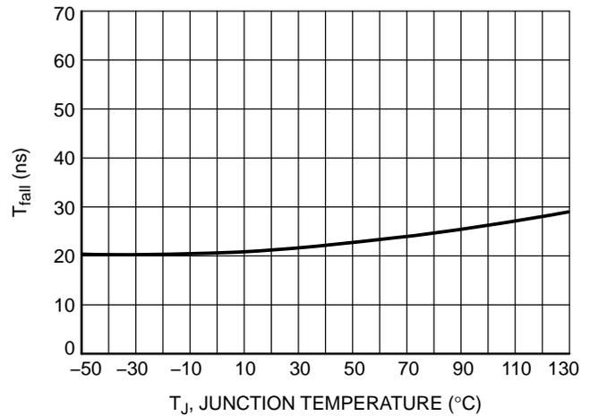
Figure 20. DRV Voltage Fall-time (C<sub>L</sub> = 1 nF, 10–90% of Output Signal) vs. Temperature
