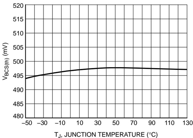
Figure 27. Current Sense Voltage Threshold vs. Temperature
