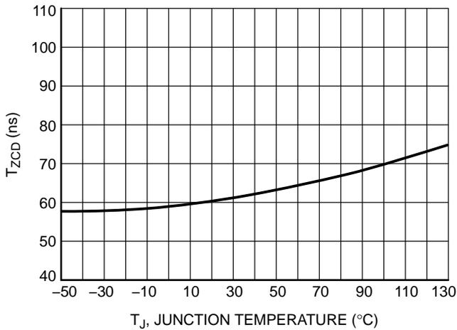
Figure 39. ((V<sub>CS/ZCD</sub> < V<sub>ZCD(th)</sub>) to DRV High) Delay vs. Temperature
