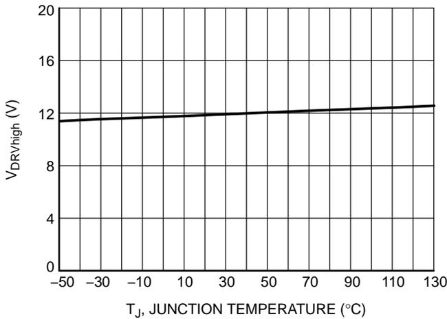
Figure 21. DRV Pin Level @ V<sub>CC</sub> = 35 V (R<sub>L</sub> = 33 kΩ, C<sub>L</sub> = 1 nF) vs. Temperature
