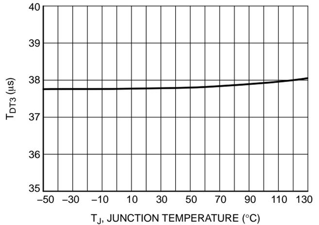
Figure 14. Dead-time,  $V_{FFcontrol} = 1.00\text{ V}$  vs. Temperature
