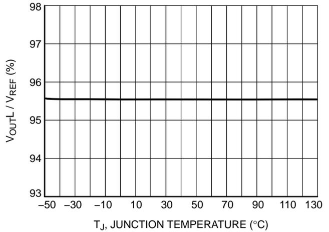
Figure 24. Ratio (V<sub>OUT</sub> Low Detect Threshold / V<sub>REF</sub>) vs. Temperature
