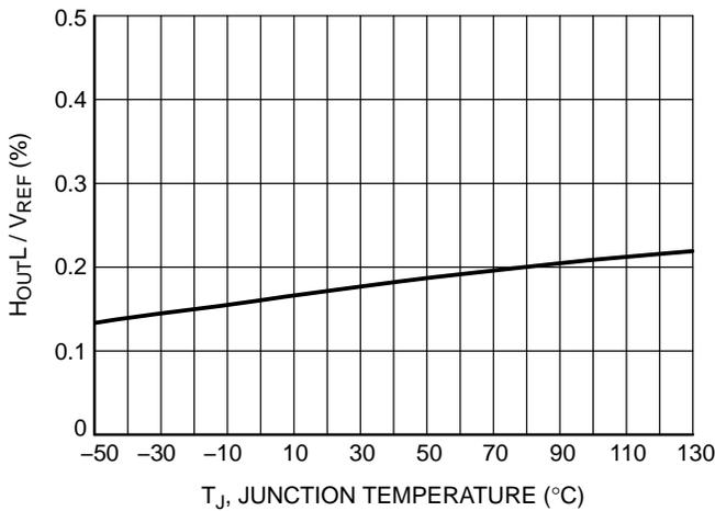
Figure 25. Ratio (V<sub>OUT</sub> Low Detect Hysteresis / V<sub>REF</sub>) vs. Temperature
