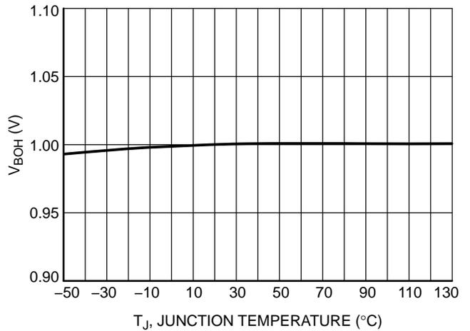
Figure 52. Brown-out Threshold,  $V_{SENSE}$  Rising vs. Temperature
