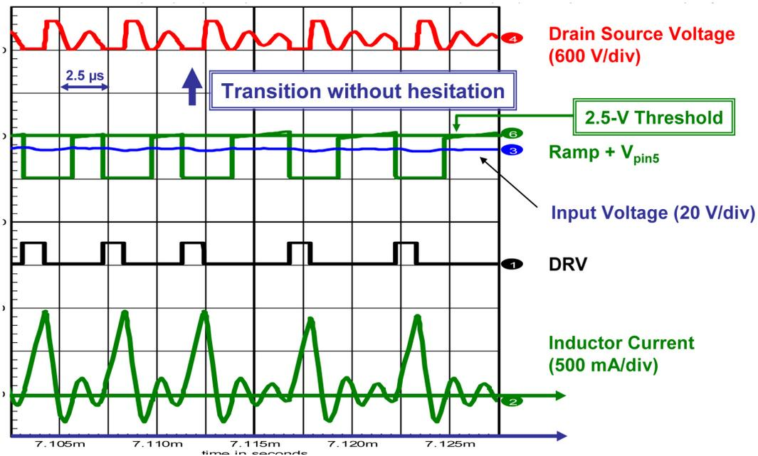
Figure 65. Clean Transition Without Hesitation Between Valleys
