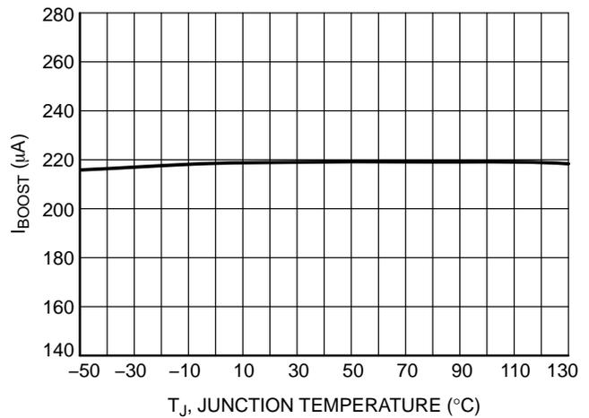
Figure 26. V<sub>CONTROL</sub> Source Current when (V<sub>OUT</sub> Low Detect) is Activated for Dynamic Response Enhancer (DRE) vs. Temperature
