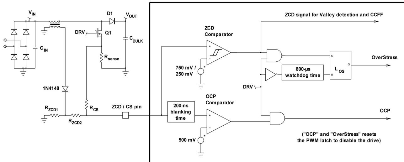
Figure 71. Current Sense and Zero Current Detection Blocks
