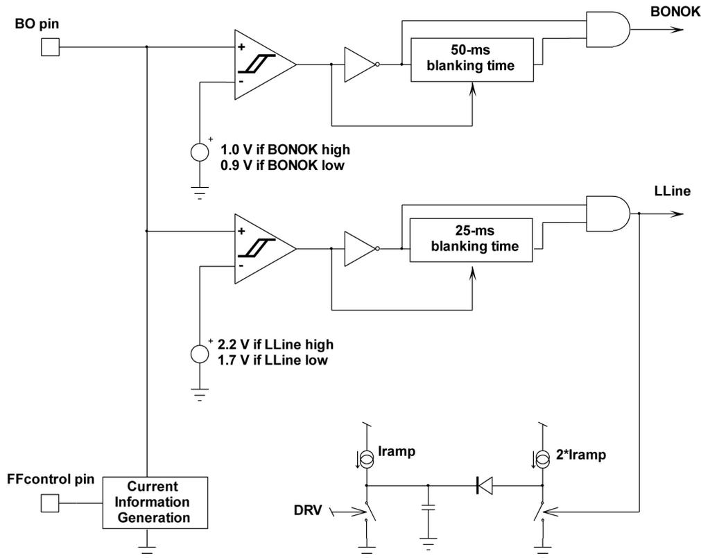
Figure 73. Input Line Sense Monitoring
