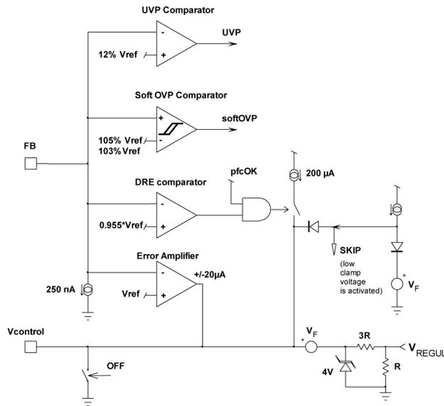
Hence,  $V_{pin3}$  features a 4 V voltage swing.  $V_{pin3}$  is then offset down by ( $V_F$ ) and scaled down by a resistors divider before it connects to the “ $V_{TON}$  processing block” and the PWM section. Finally, the output of the regulation block is a signal (“ $V_{REGUL}$ ” of the block diagram) that varies between 0 and a top value corresponding to the maximum on-time.
