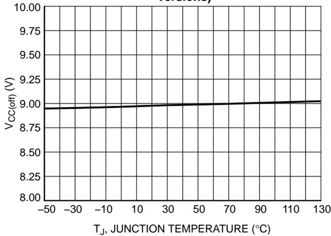
Figure 7. V<sub>CC</sub> Minimum Operating Voltage, V<sub>CC</sub> Falling (V<sub>CC(off)</sub>) vs. Temperature
