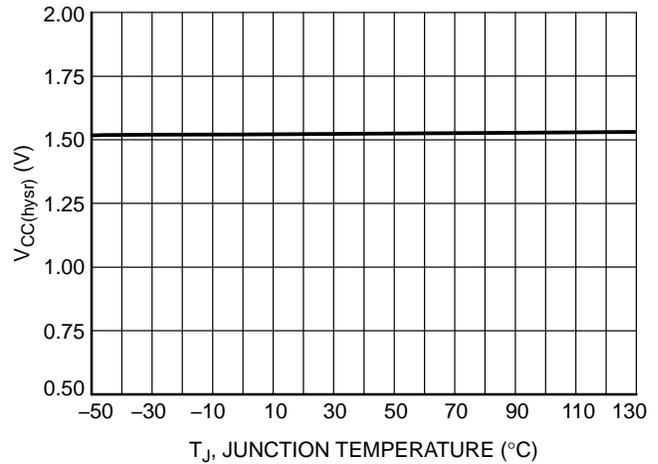
Figure 8. Hysteresis (V<sub>CC(on)</sub> - V<sub>CC(off)</sub>) vs. Temperature (A, A1, A2 and A3 Versions)
