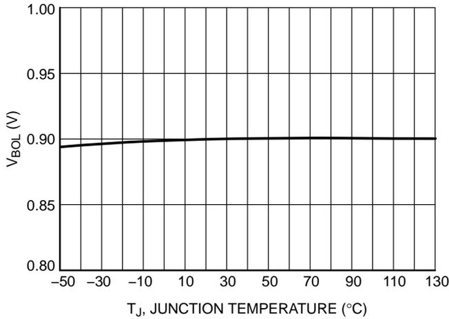
Figure 53. Brown-out Threshold,  $V_{SENSE}$  Falling vs. Temperature
