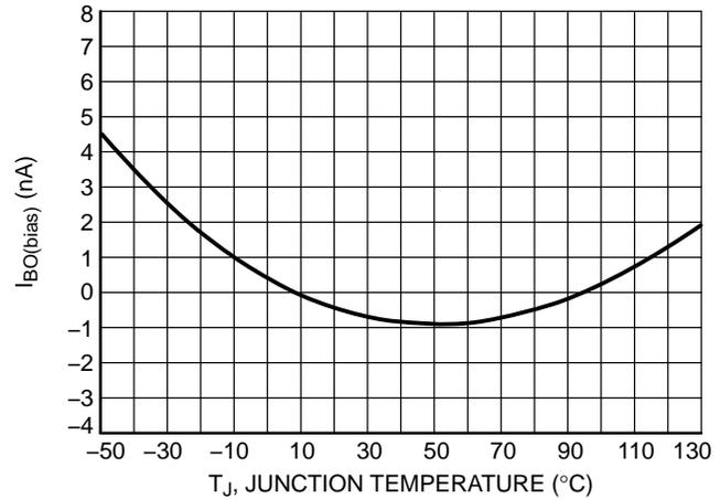
Figure 60. Brown-out Pin Bias Current, (V<sub>SENSE</sub> = V<sub>BOH</sub>) vs. Temperature
