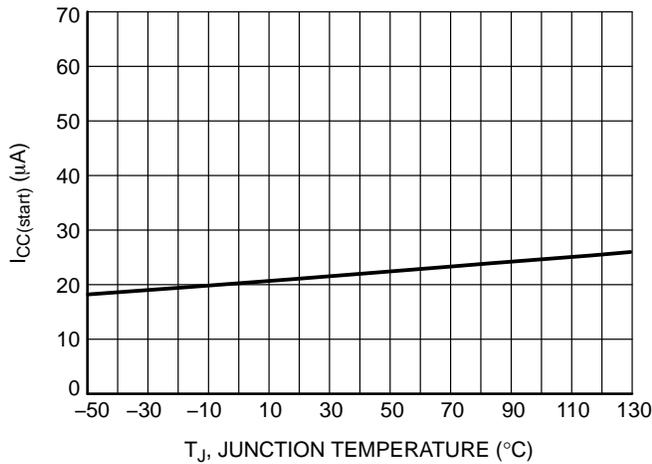
Figure 9. Start-up Current @ V<sub>CC</sub> = 9.4 V vs. Temperature
