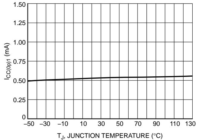
Figure 10. Operating Current, No Switching (V<sub>SENSE</sub> Grounded) vs. Temperature
