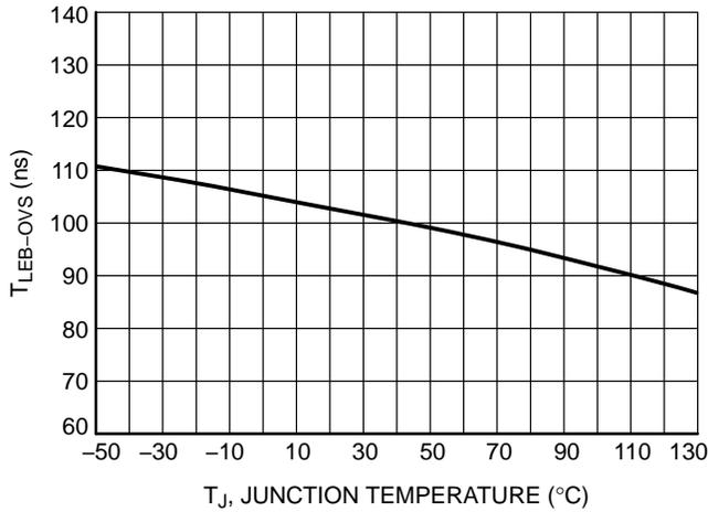
Figure 29. “Overstress” Protection Leading Edge Blanking vs. Temperature
