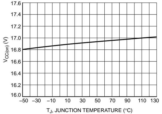
Figure 6. Start-up Threshold, V<sub>CC</sub> Increasing (V<sub>CC(on)</sub>) vs. Temperature (B and B2 Versions)
