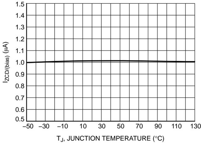
Figure 35. CS/ZCD Pin Bias Current @ V<sub>CS/ZCD</sub> = 0.75 V vs. Temperature
