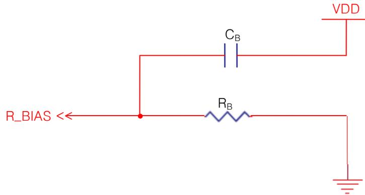
The R\_BIAS is connected to the resistor to decide the oscillator and internal bias current. The sensing frequency, internal clock frequency and current consumption are therefore able to be adjusted with R<sub>B</sub>. A voltage ripple on R\_BIAS can make critical internal error, so C<sub>B</sub> connected to the VDD (not GND) is recommended. (The typical value of C<sub>B</sub> is 820pF and the maximum Value is 1nF.)
