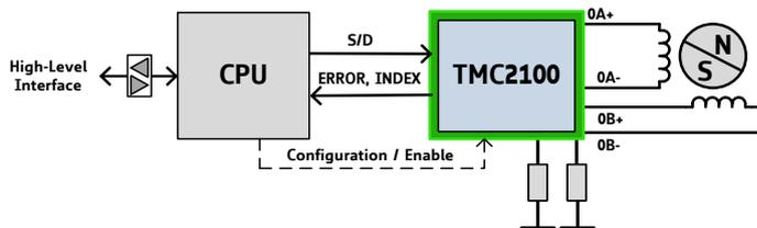
Here, the CPU sends step and direction signals to the TMC2100 and reads out ERROR and INDEX for diagnostic tasks. Further, the CPU configures the TMC2100 and manages motion control. Based on Step/Dir signals, the TMC2100 provides motor currents for each axis and smoothens and optimizes drive performance.
