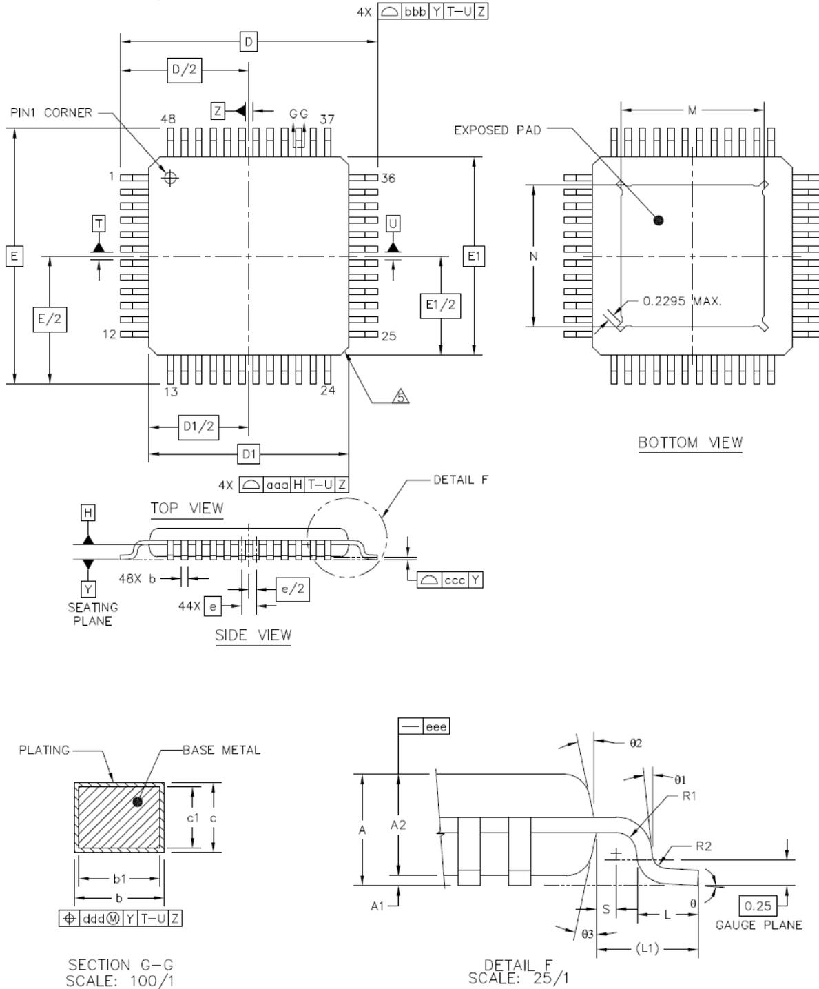
Figure 17.2 Dimensional drawings TQFP-EP48
