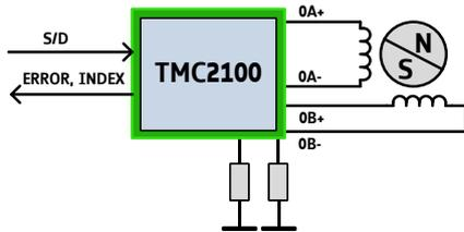
In this example, configuration is hard wired. The motor is driven via step and direction signals. Motion control tasks and interpreting ERROR and INDEX are software based.
