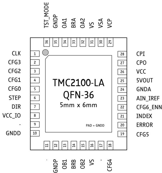
Figure 2.1 TMC2100-LA package and pinning QFN-36 (5x6mm<sup>2</sup>)
