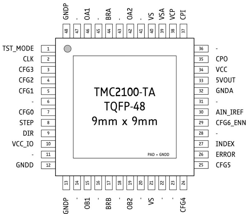
Figure 2.2 TMC2100-TA package and pinning TQFP-48 (9x9mm<sup>2</sup> with leads)
