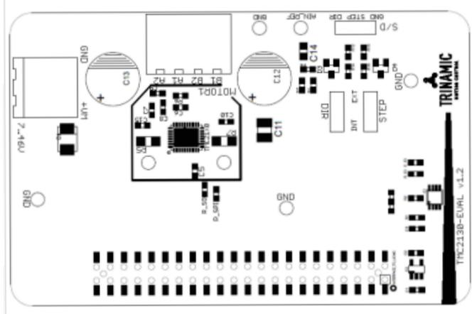
The TMC2100-EVAL is part of TRINAMICs universal evaluation board system which provides a convenient handling of the hardware as well as a user-friendly software tool for evaluation. The TMC2100 evaluation board system consists of three parts: STARTRAMPE (base board), ESELSBRÜCKE (connector board with several test points), and TMC2100-EVAL.
