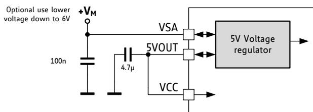
**Figure 4.1** Reduced number of filtering components
