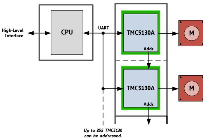
An application with 2 stepper motors is shown. Additionally, the ABN Encoder interface and two reference switches can be used for each motor. A single CPU controls the whole system. The CPU-board and the controller / driver boards are highly economical and space saving.
