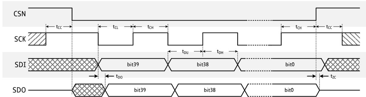
**Figure 4.1 SPI timing**
