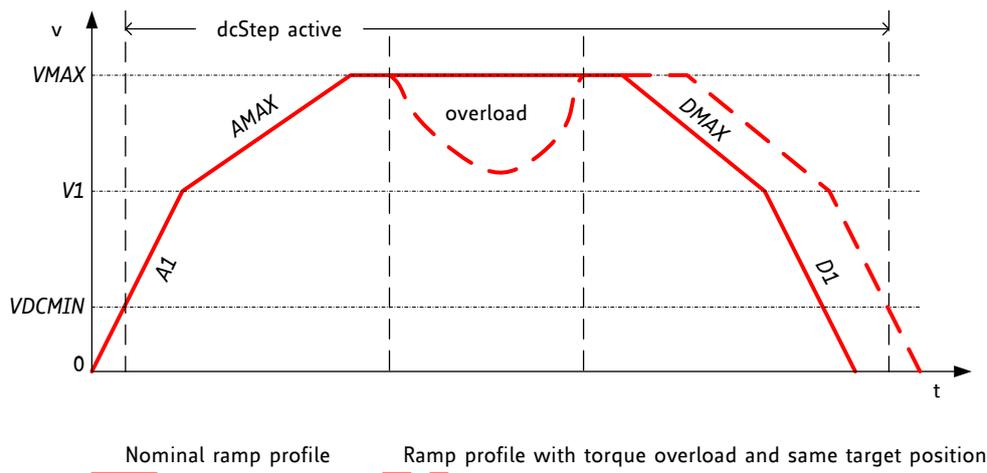
Figure 19.2 Velocity profile with impact by overload situation
