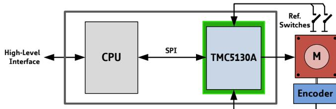
An ABN encoder interface with scaler unit and two reference switch inputs are used to control motor movement.
