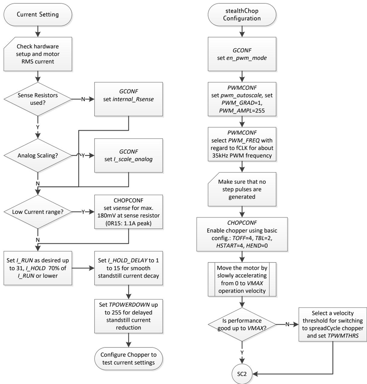
Figure 24.1 Current setting and first steps with StealthChop
