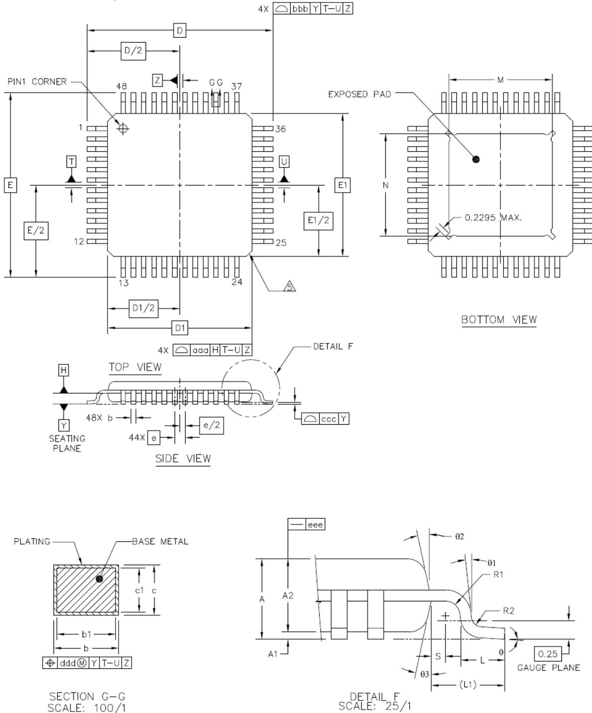
Figure 32.1 Dimensional drawings TQFP48-EP
