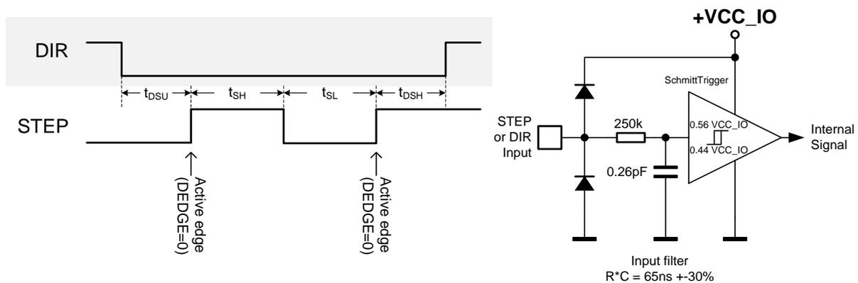
Figure 17.1 STEP and DIR timing, Input pin filter
