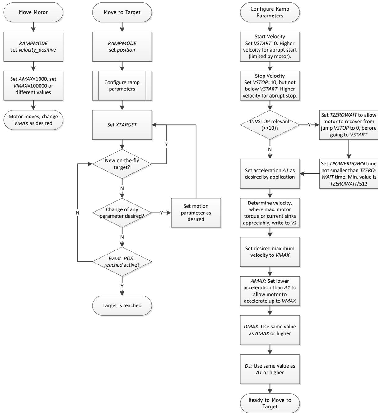
**Figure 24.3** Moving the motor using the motion controller
