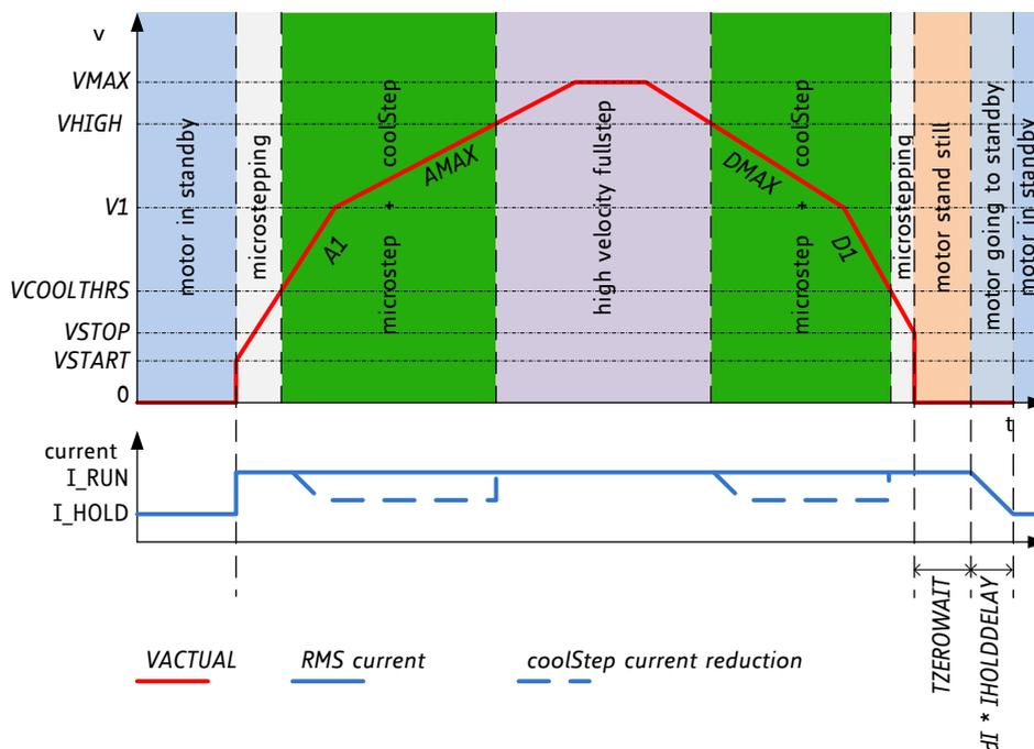
Figure 14.3 Ramp generator velocity dependent motor control
