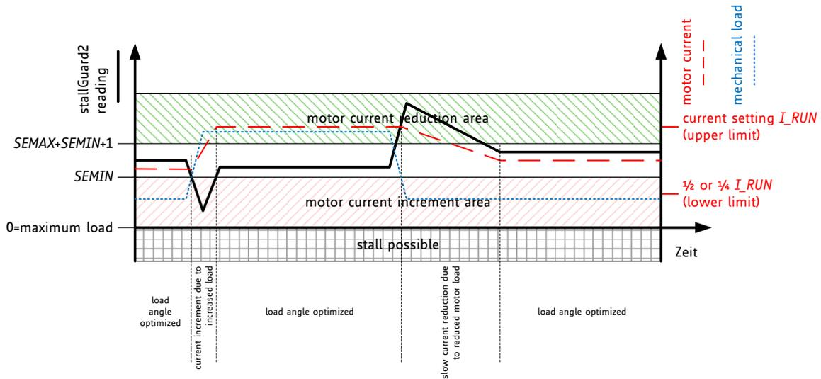
**Figure 16.1 CoolStep adapts motor current to the load**
