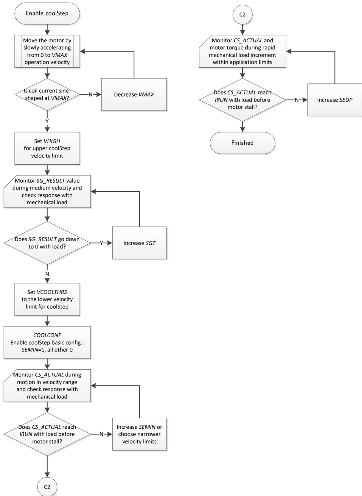
**Figure 18.4 Enabling coolStep (only in combination with spreadCycle)**
