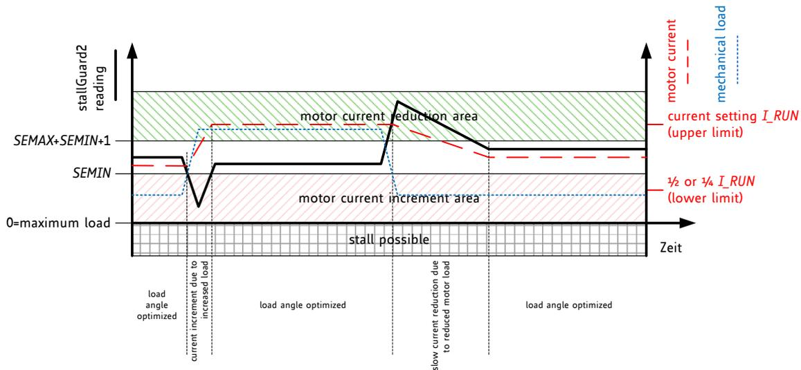
**Figure 13.1 coolStep adapts motor current to the load**
