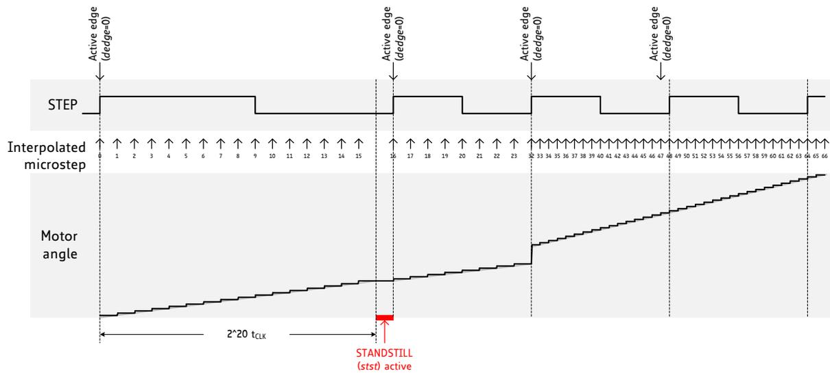
**Figure 16.2** microPlyer microstep interpolation with rising STEP frequency
