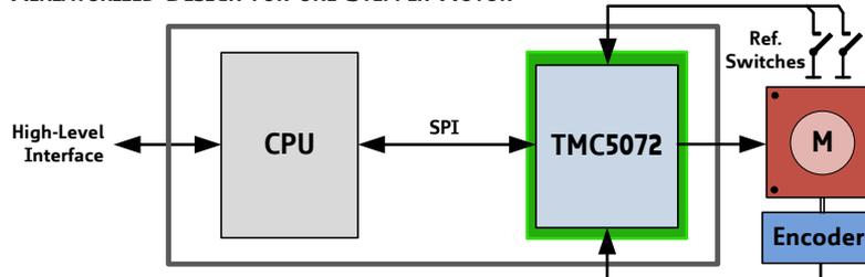
The stepper motor driver outputs are switched in parallel. A dual ABN encoder interface and two reference switch inputs are used.
