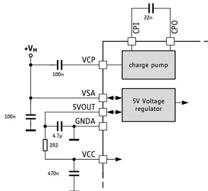
Figure 3.6 RC-Filter on VCC for reduced ripple
