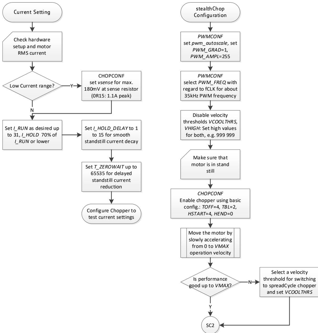
Figure 18.1 Current setting and first steps with stealthChop
