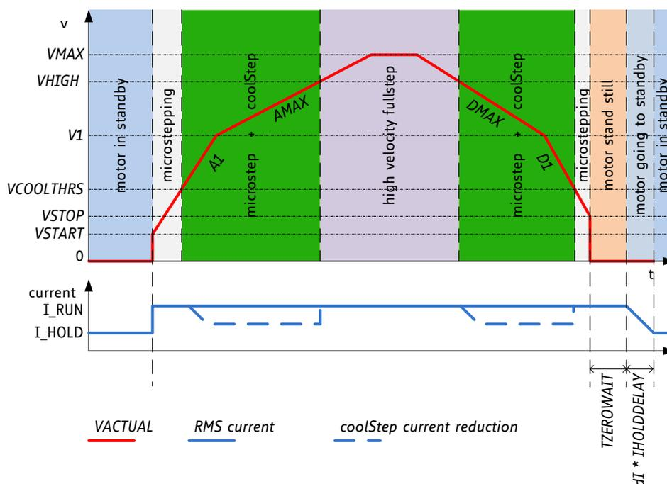
Figure 11.3 Ramp generator velocity dependent motor control
