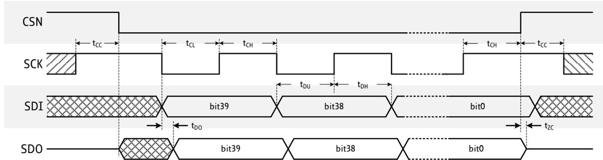
**Figure 4.1** SPI timing
