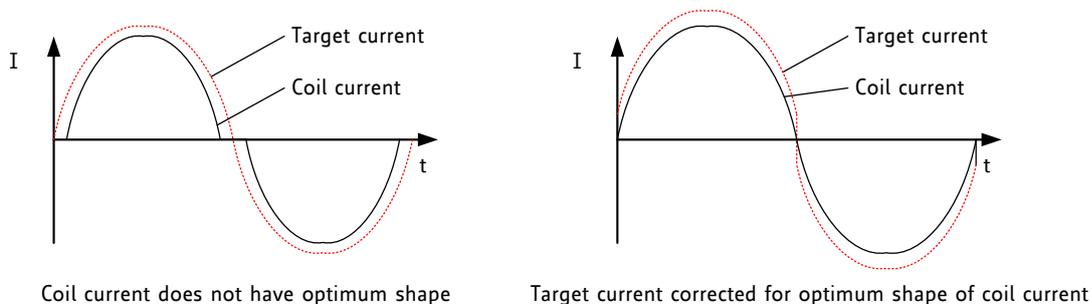
**Figure 9.5 Zero crossing with classic chopper and correction using sine wave offset**
