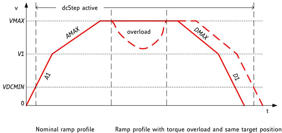
**Figure 14.2 Velocity profile with impact by overload situation**
