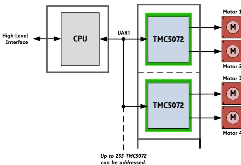
An application for up to 510 stepper motors is shown. The UART single wire differential interface allows for a decentralized distributed system with a minimized number of components. Additionally, an ABN encoder and up to two reference switches can be used for each motor. A single CPU can control the whole system. The CPU-board and controller / driver boards are highly economical and space saving.
