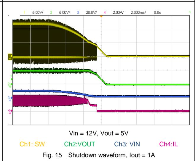
Fig. 15 Shutdown waveform, Iout = 1A
