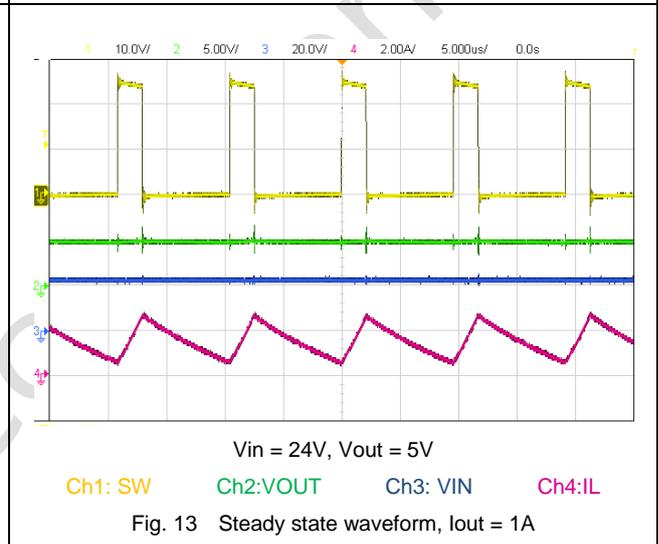
Fig. 13 Steady state waveform, Iout = 1A
