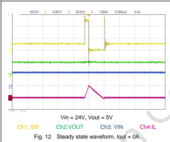
Fig. 12 Steady state waveform, Iout = 0A
