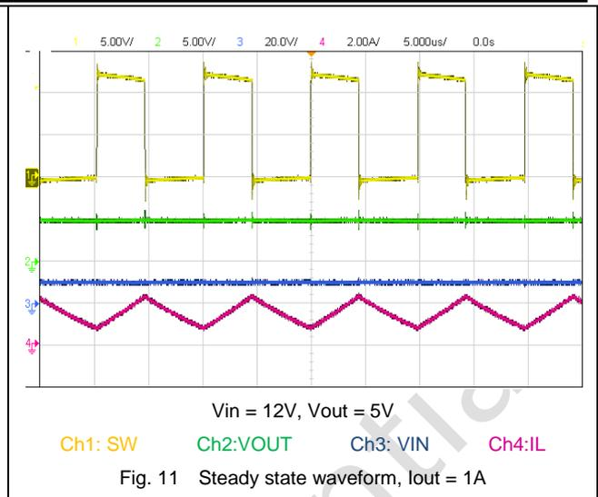
Fig. 11 Steady state waveform, Iout = 1A
