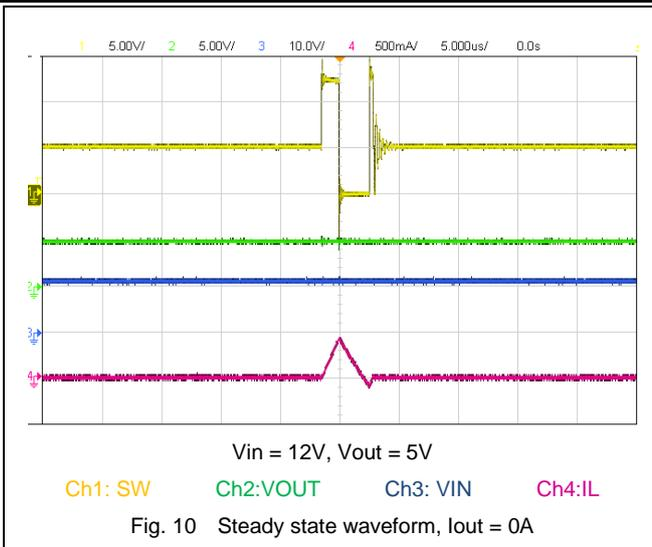
Fig. 10 Steady state waveform, Iout = 0A
