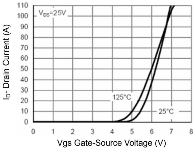
Figure 2 Transfer Characteristics
