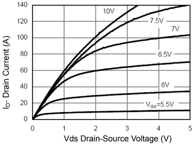
Figure 1 Output Characteristics
