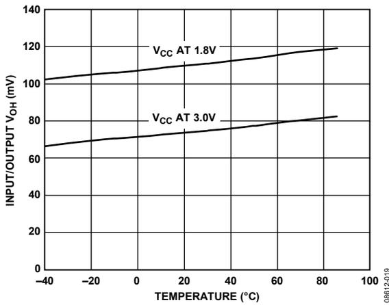
Figure 6. Input/Output V<sub>OH</sub> vs. Temperature (Source Current = 1 mA)
