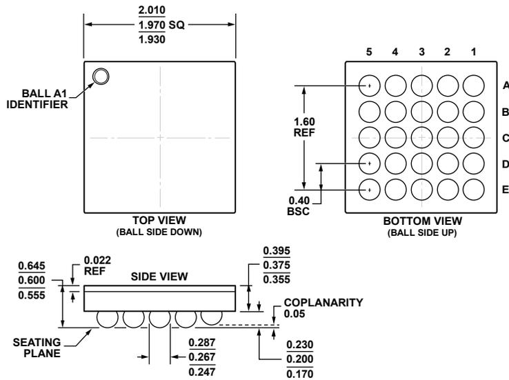
Figure 22. 25-Ball Wafer Level Chip Scale Package [WLC]
