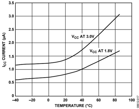
Figure 5. Standby (I<sub>CC</sub>) Current vs. Temperature
