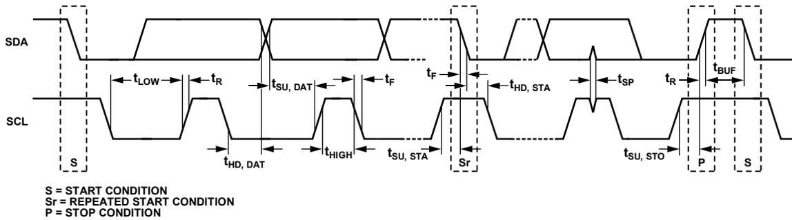
Figure 2. I<sup>2</sup>C Interface Timing Diagram
