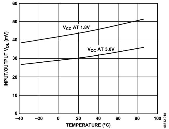
Figure 7. Input/Output V<sub>OL</sub> vs. Temperature (Sink Current = 1 mA)
