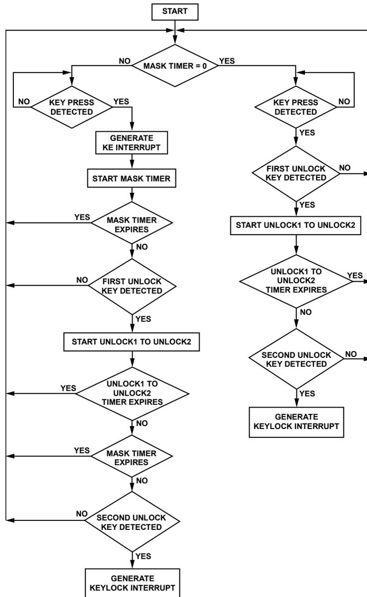
Figure 12. Keypad Lock Interrupt Mask Timer Flowchart
