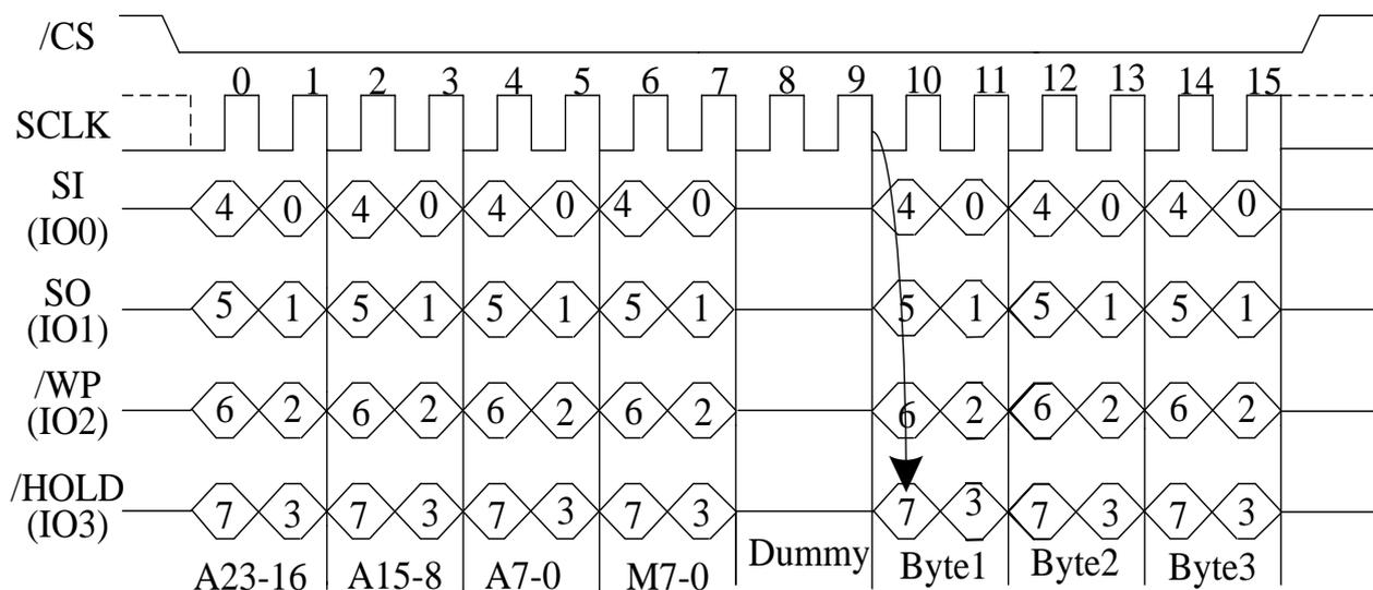
**Quad I/O Word Fast Read with “8/16/32/64-Byte Wrap Around” in standard SPI mode**
