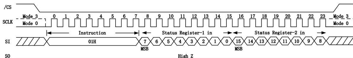
Figure 8.b. Write Status Register-1/2 Instruction (QPI Mode)
