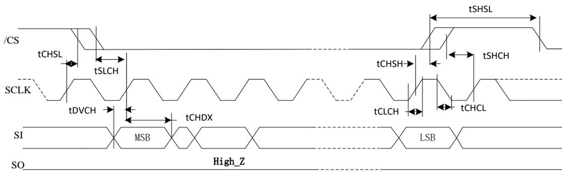
Figure 47. Output Timing
