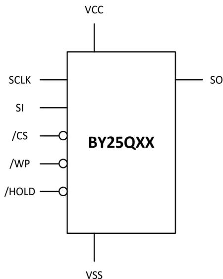
Figure 2. Pin Configuration SOP 208 mil
