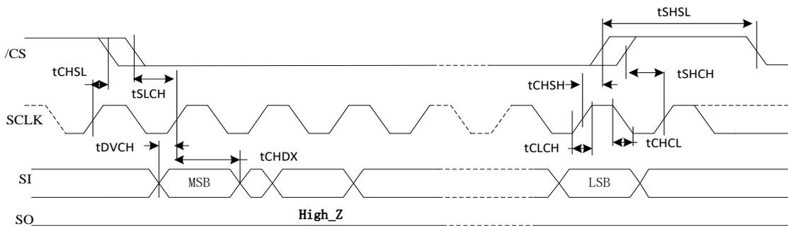
Figure 47. Output Timing
