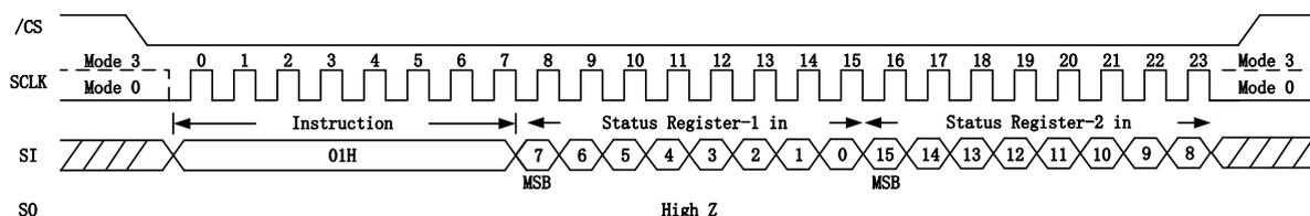
Figure 8.d. Write Status Register-1/2 Instruction (QPI Mode)
