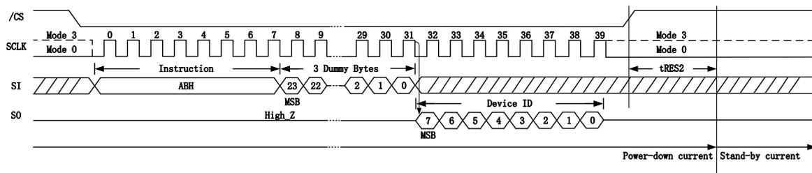
Figure 26.d. Release Power-down / Device ID Instruction (QPI Mode)
