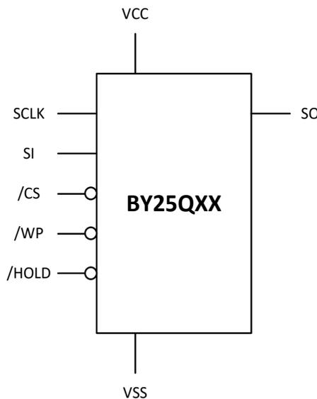
Figure 2. Pin Configuration SOP8
