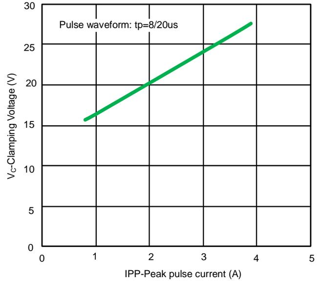
Fig 4. Clamping voltage vs. Peak pulse current
