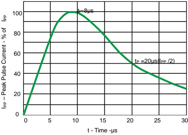
Fig 1. Pulse Waveform
