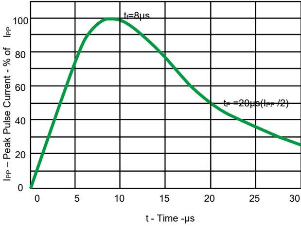
Fig 1. Pulse Waveform
