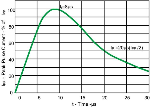
Fig 1. Pulse Waveform
