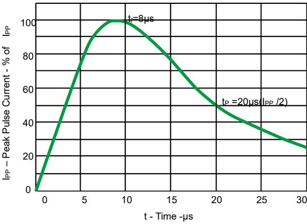
Fig 1. Pulse Waveform
