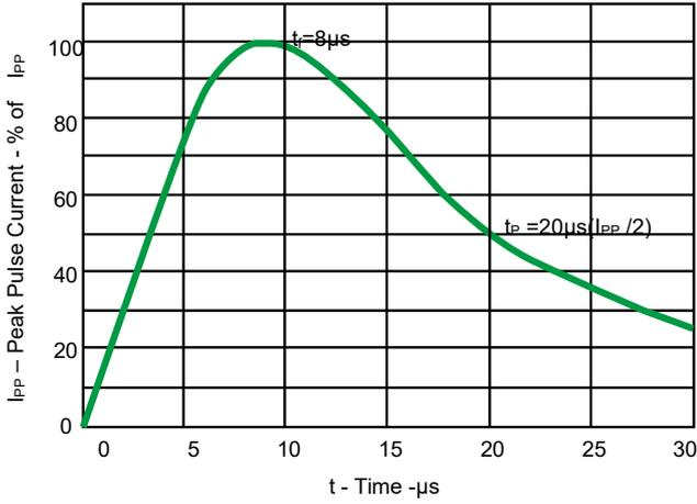
Fig 1. Pulse Waveform
